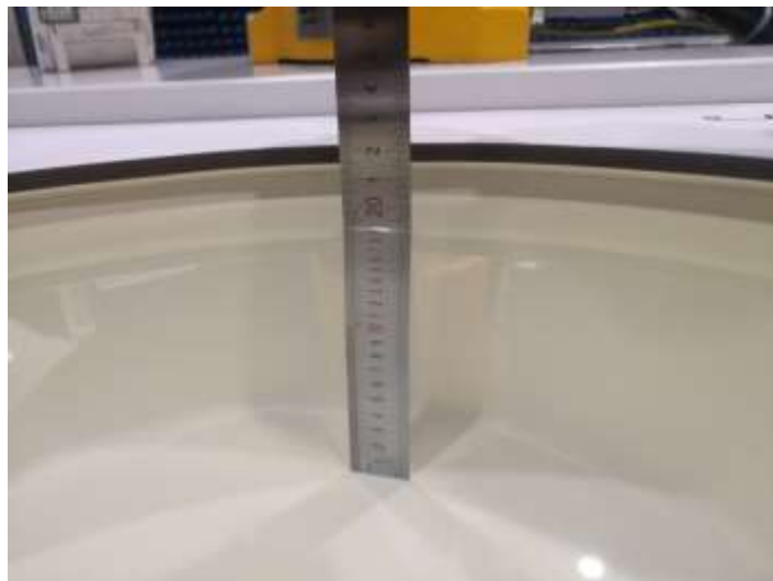
Fig. 9.2 Photo of Liquid Height for Body SAR of Twin Phantom (5000MHz~5800MHz) (depth>15cm)
