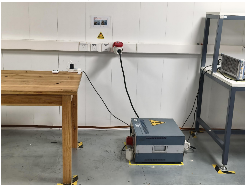
Test Setup Photo(s) of Conducted Emissions Measurement
