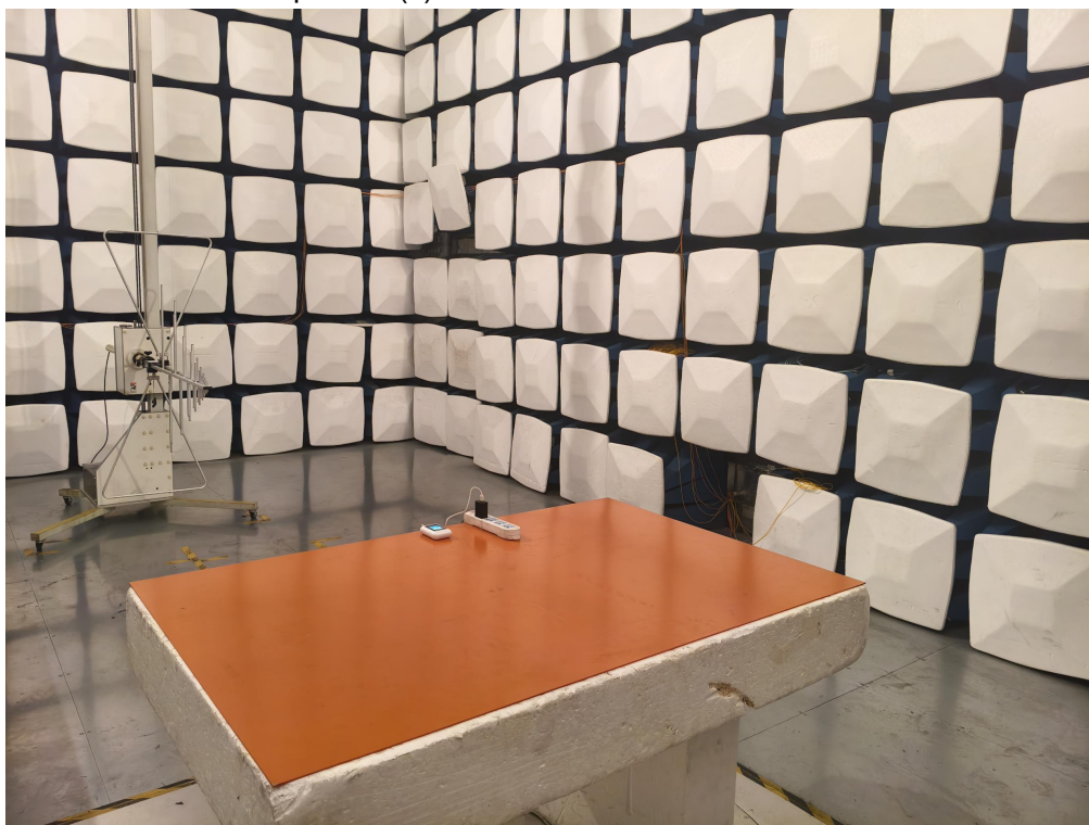
Test Setup Photo(s) of Radiated Emissions Measurement
