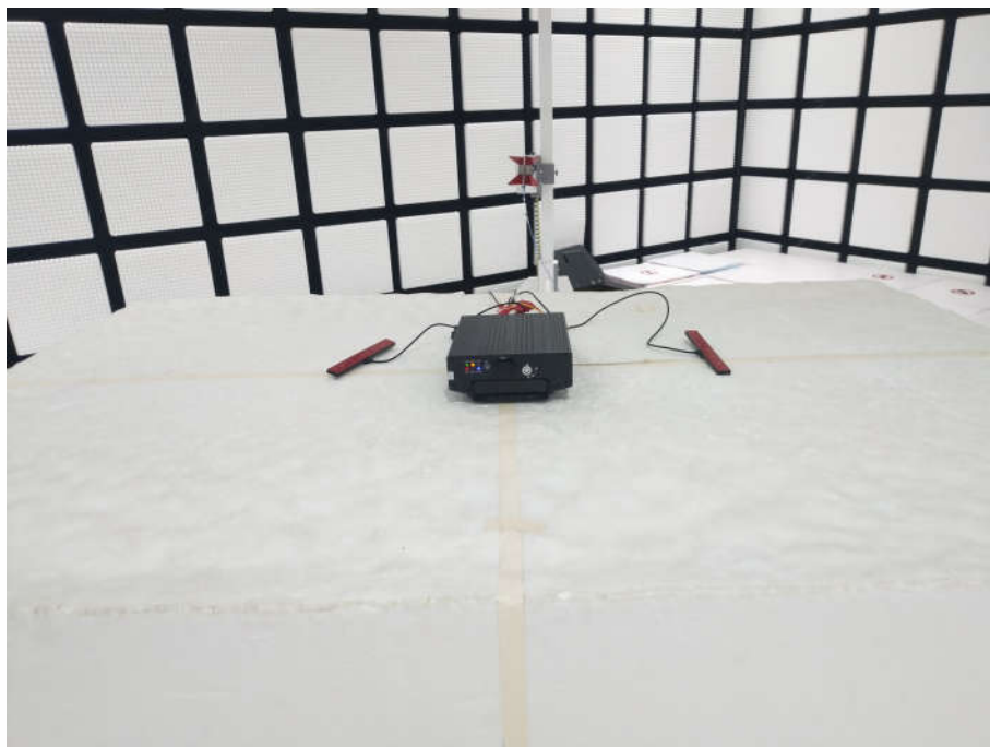
Radiated spurious emission Test Setup-3(Above 1GHz)
