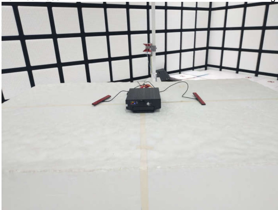
Radiated spurious emission Test Setup-3(Above 1GHz)
