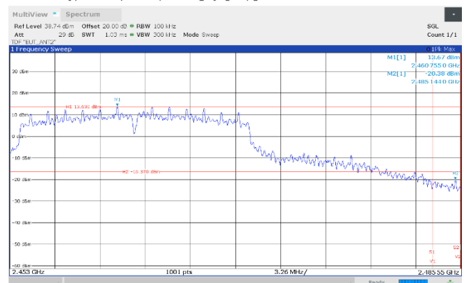
Figure 8.7-20: Authorized band-edge emissions, 2462 MHz, Antenna 2
