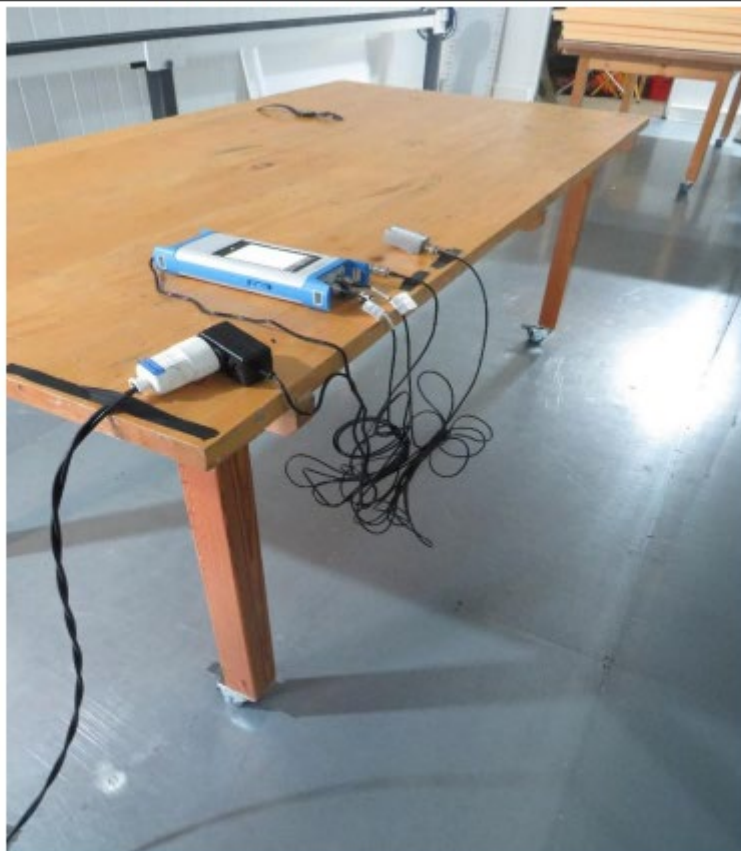
Setup for measurements 150 kHz – 30 MHz
