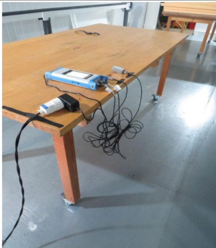
Setup for measurements 150 kHz – 30 MHz
