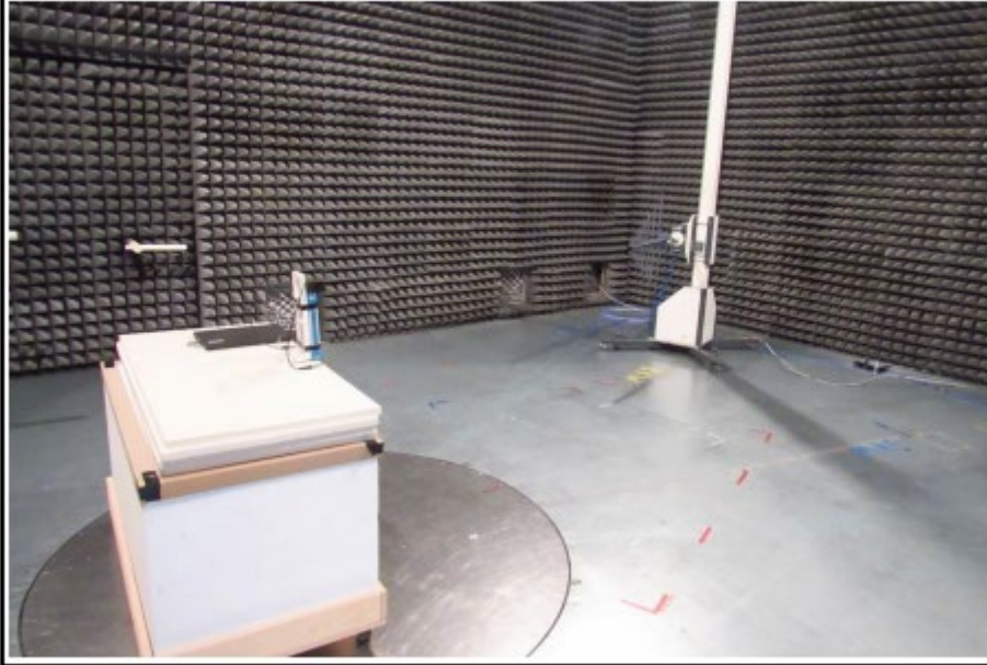
Setup for measurements below 1 GHz
