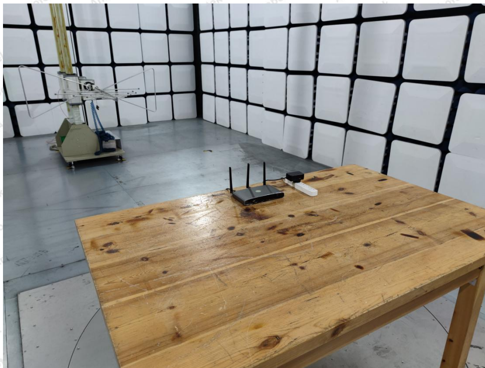
Photo of Radiation Emission Test
