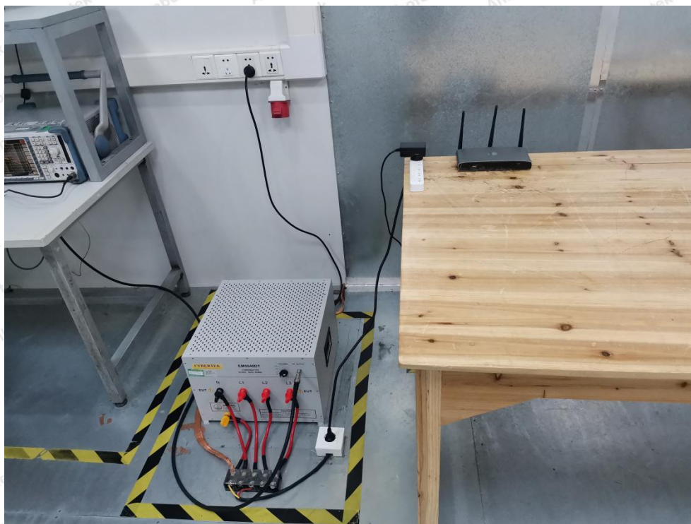
Photo of Conducted Emission Test
