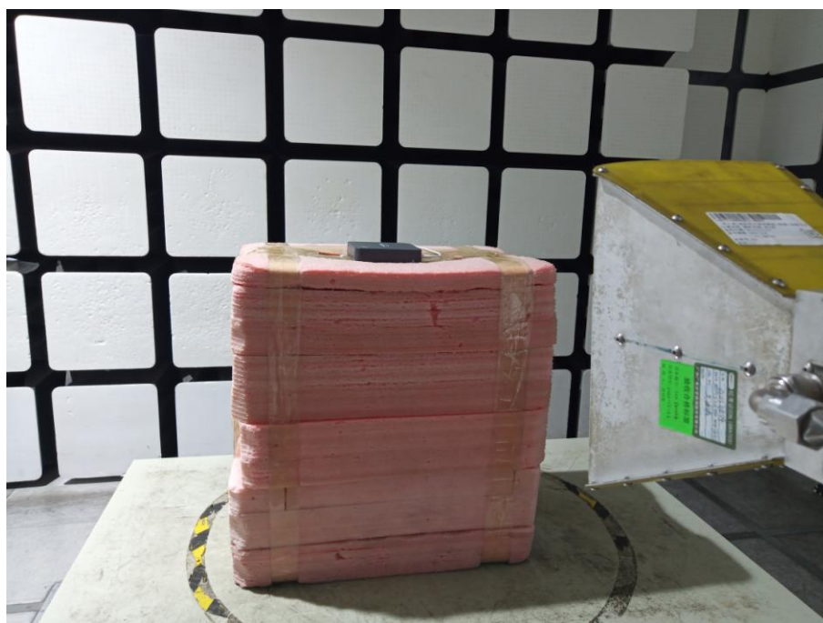
Radiated Emissions View (Above 1 GHz, 1m)
