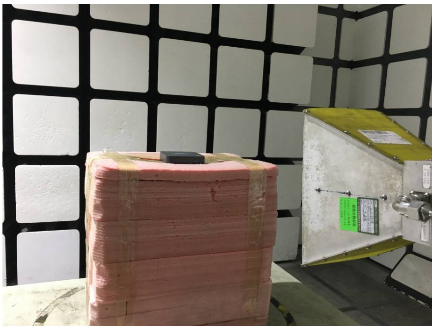
Radiated Emissions View (Above 1 GHz, 1m)
