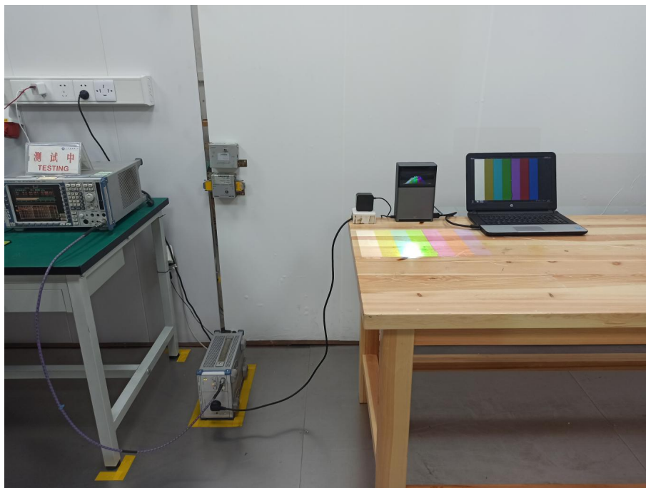
Conducted Emissions Test Setup
