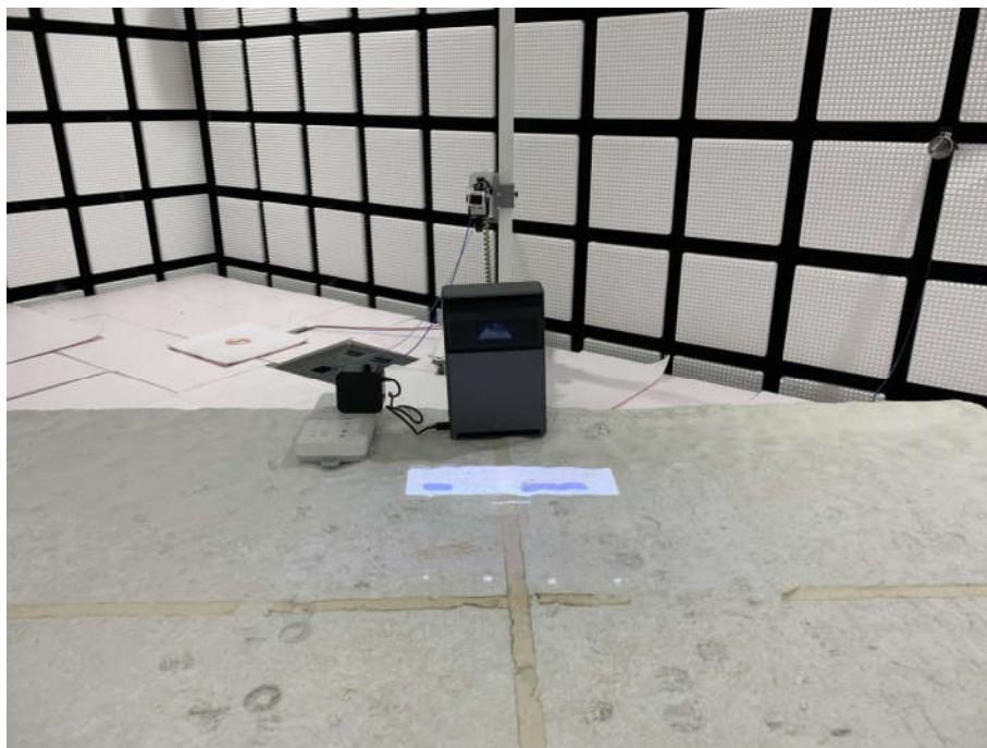
Radiated spurious emission Test Setup-5(Above 18GHz)
