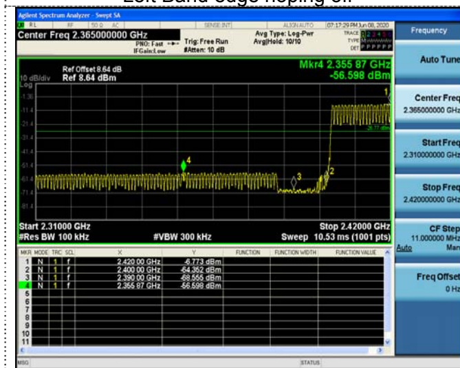
Left Band edge hopping on
