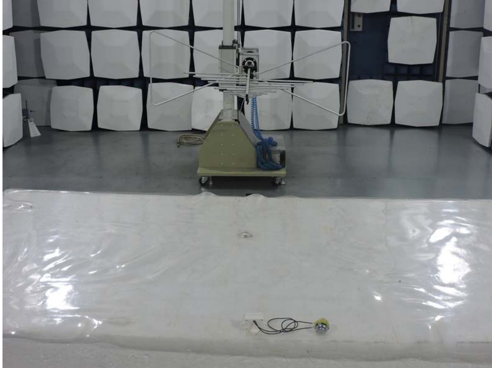
Radiated Emission Test Setup:
