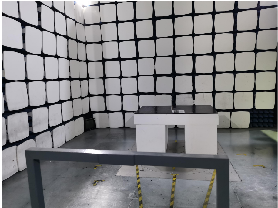
Radiation Emission Test Setup (Below 30MHz)
