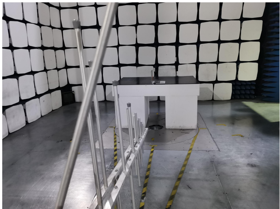
Radiation Emission Test Setup (30MHz to 1GHz)
