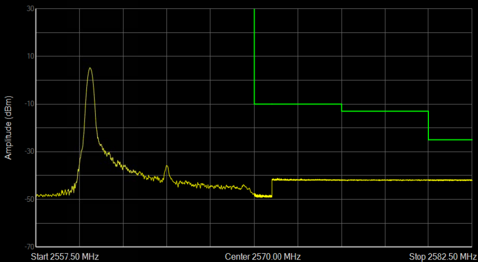
LTE Band7 QPSK BW=10MHz Channel=21400 RB Size=1 Position=#0
