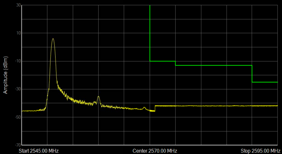
LTE Band7 QPSK BW=20MHz Channel=21350 RB Size=1 Position=#0
