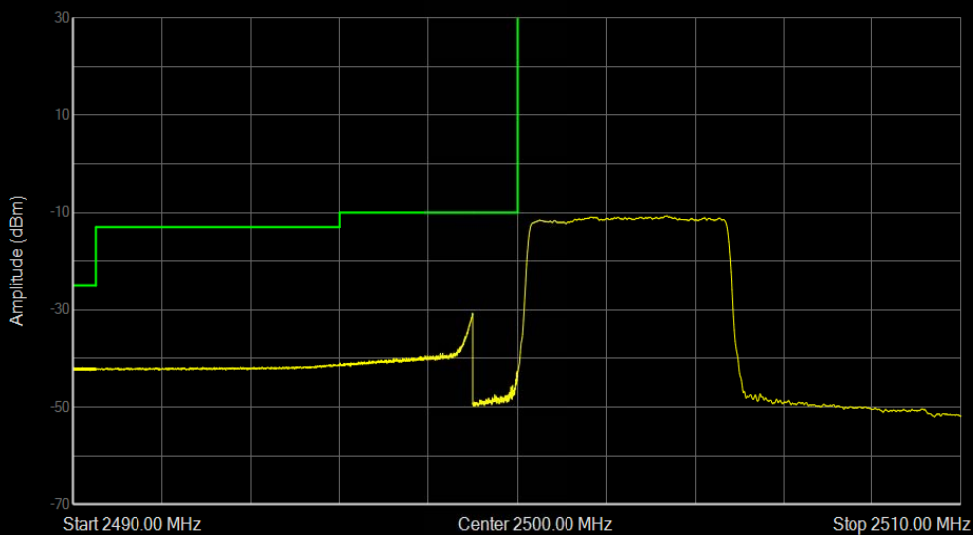
LTE Band7 QPSK BW=5MHz Channel=20775 RB Size=25 Position=#0
