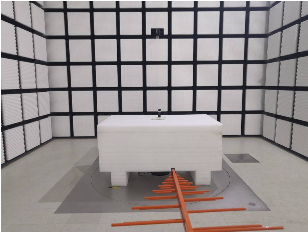
Radiated Emissions Below 1G View
