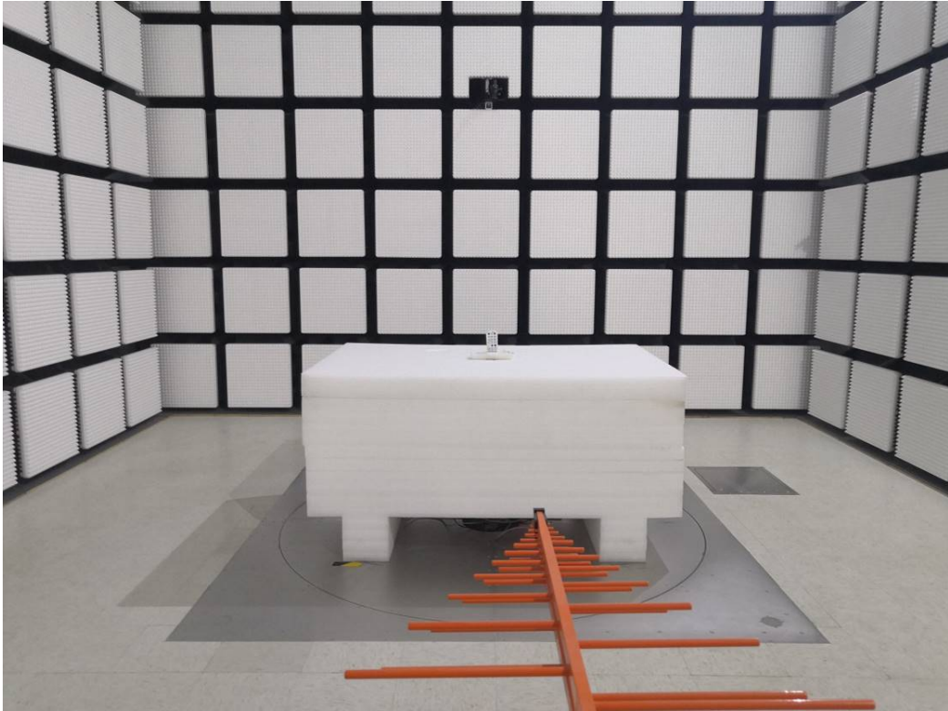
Radiated Emissions Above 1G View
