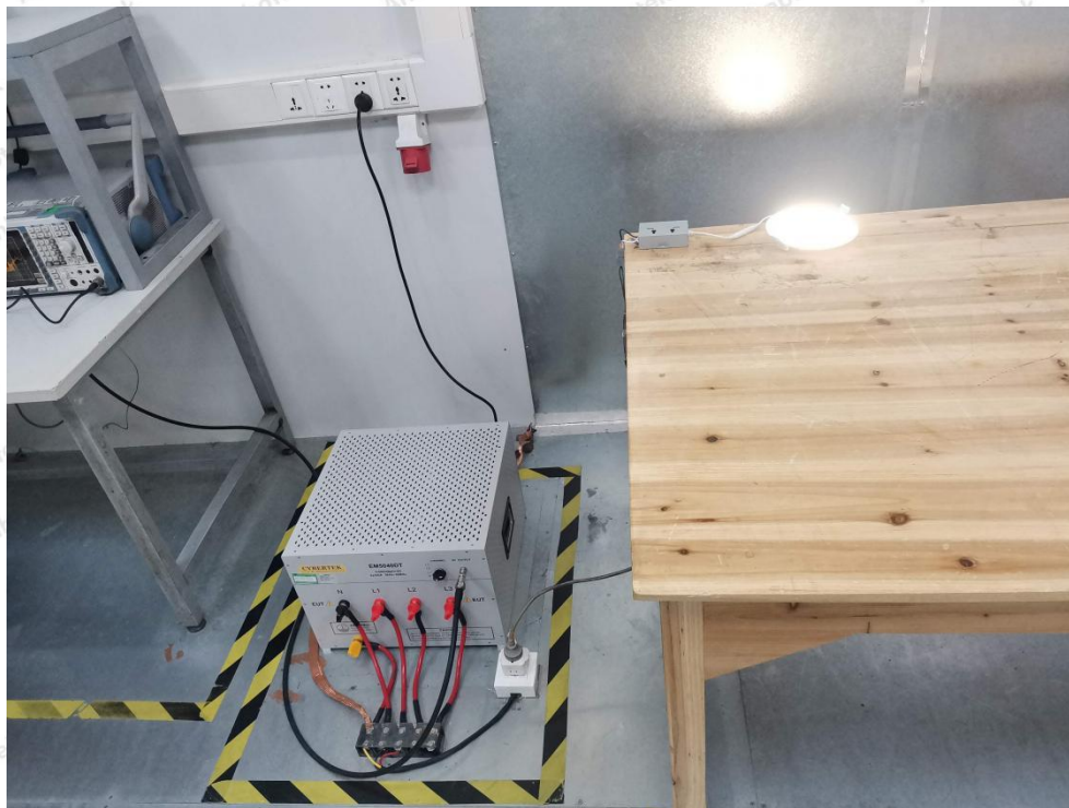
Photo of Conducted Emission Measurement
