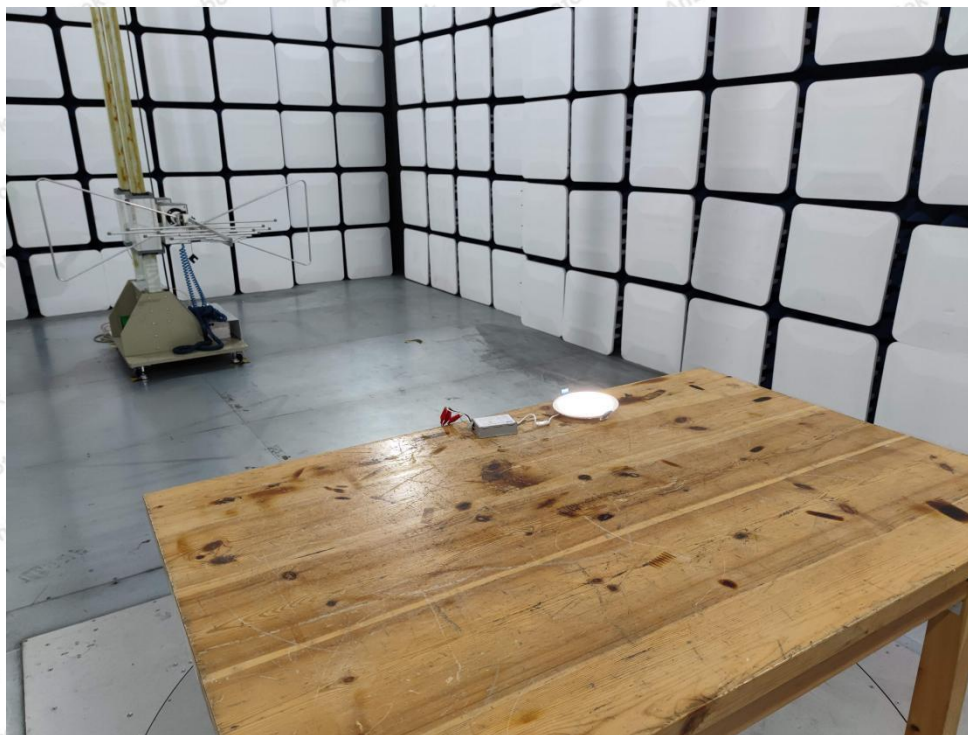
Photo of Radiation Emission Test
