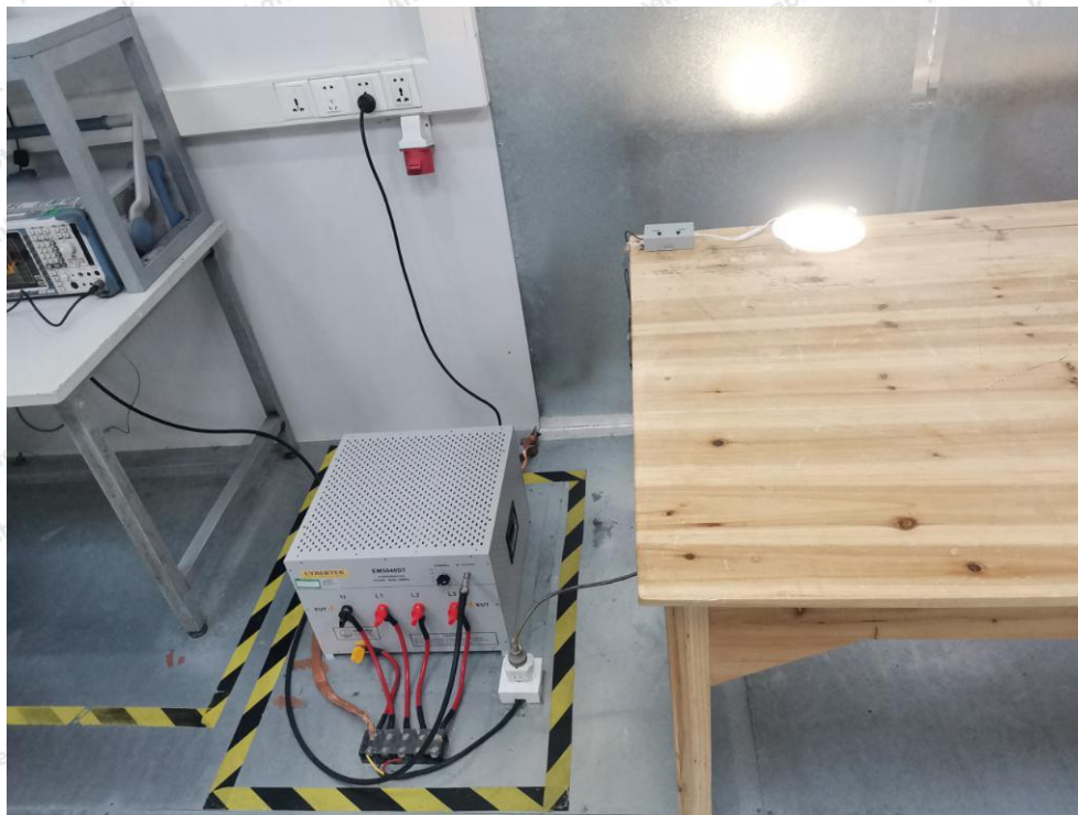
Photo of Conducted Emission Measurement
