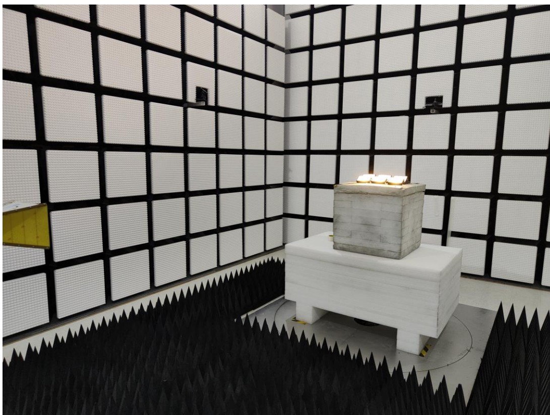
Radiated Emission Above 1GHz View
