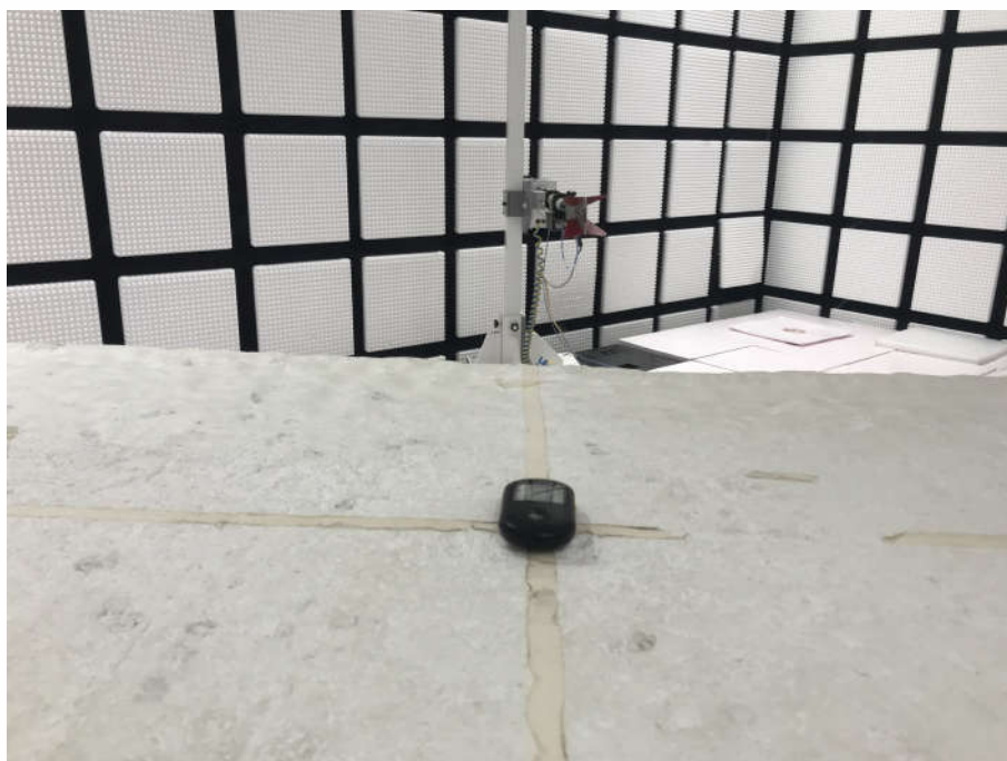
Radiated spurious emission Test Setup-2(Above 1GHz)
