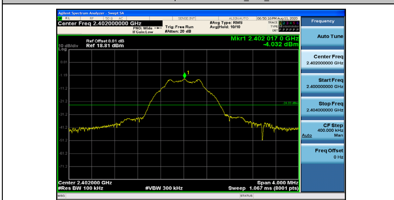
RF Conducted Spurious Emissions_BLE_2402
