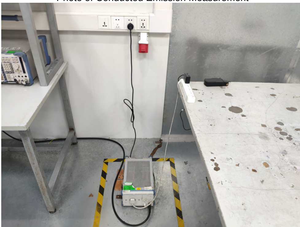
FCC ID: 2AWQV-C190POS Photo of Conducted Emission Measurement
