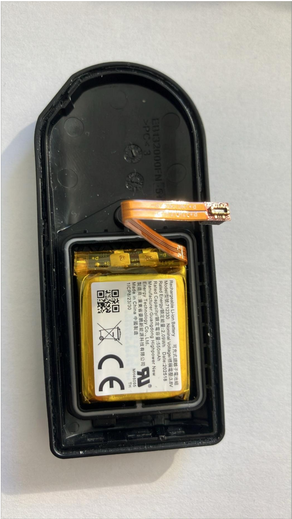
Figure 2: BCM3101 Top Cover + Battery
