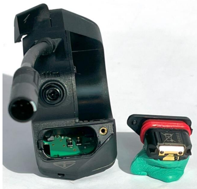
Figure 3: BRC3610 battery removed
