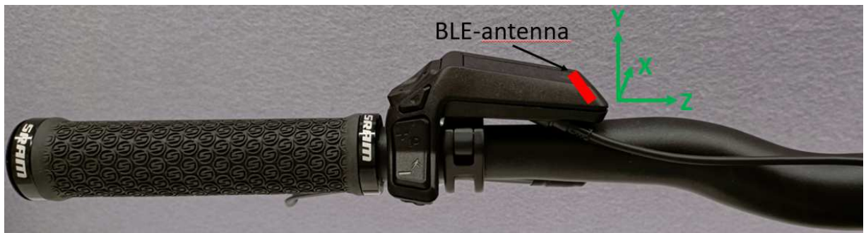
Figure 3.0. BLE-antenna positioning and orientation during to measurements.
