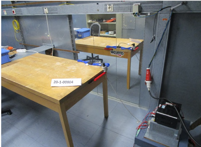
Photograph 1: EUT Test Setup for conducted emissions
