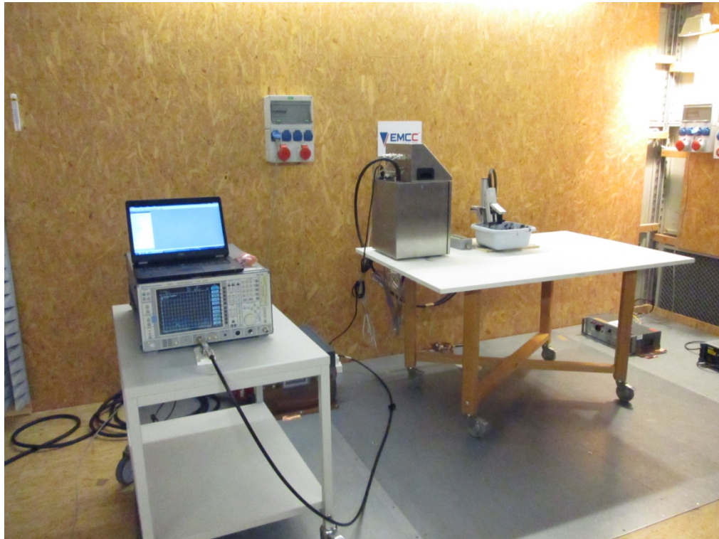
Photograph A1-1: Conducted Emissions
