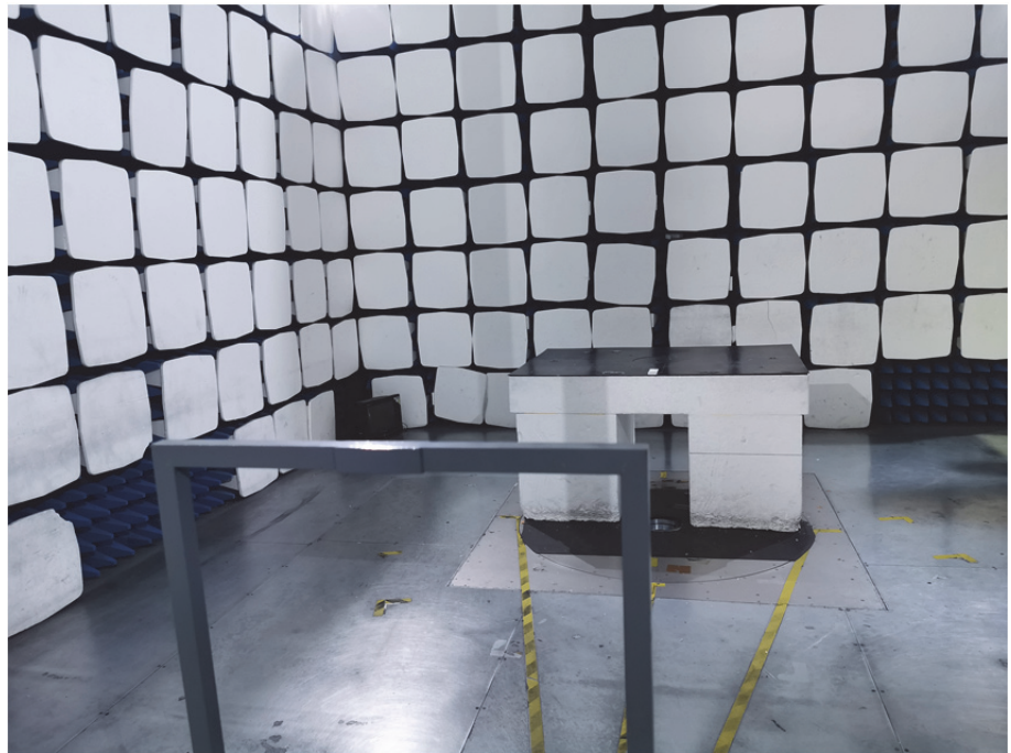
Radiation Emission Test Setup (Below 30MHz)
