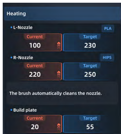
Fig. 4.45 Heating the Nozzle
