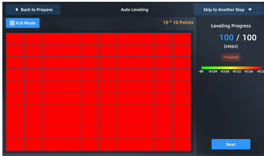
Fig. 4.50 100-Point Leveling Failed
