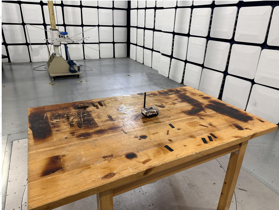
Photo of Radiation Emission Test
