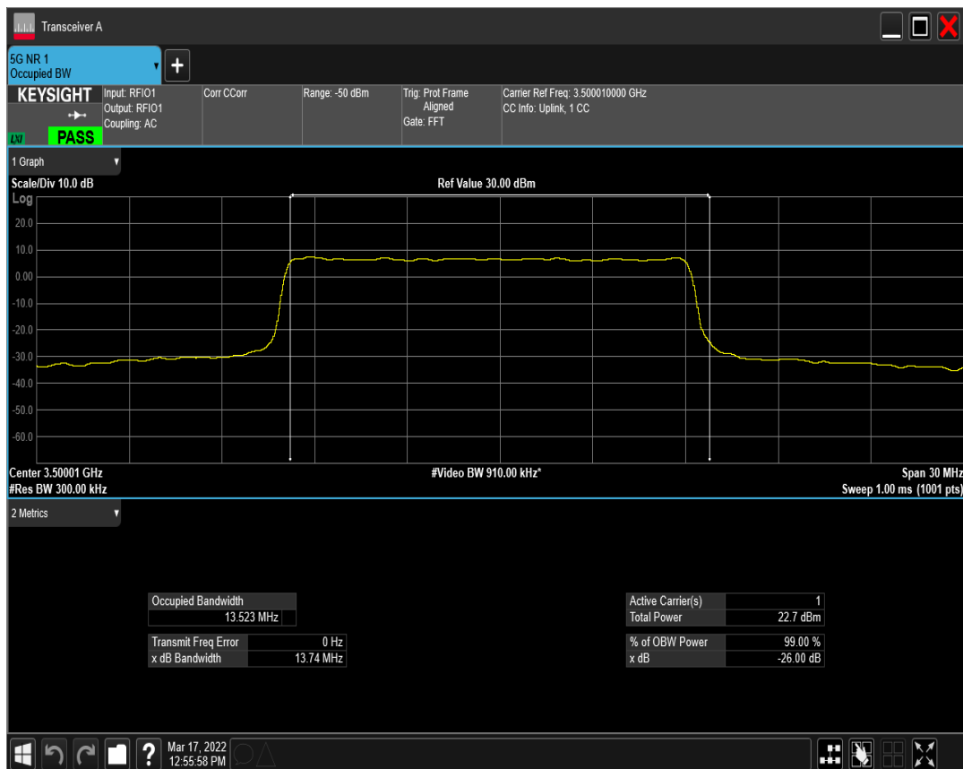
n77(3450-3550) SCS=30kHz DFT_QAM256 BW=15MHz Channel=633334 RB=36@0
