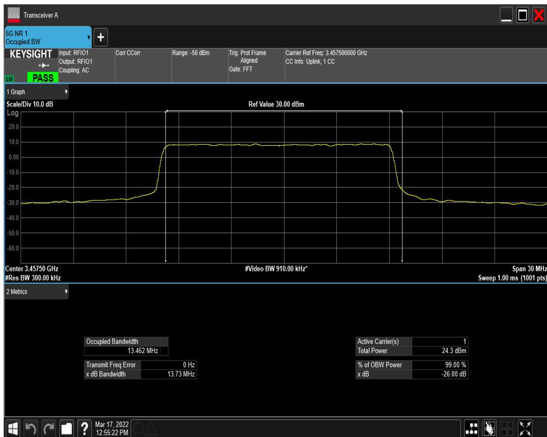
n77(3450-3550) SCS=30kHz DFT_QAM16 BW=15MHz Channel=630500 RB=36@0
