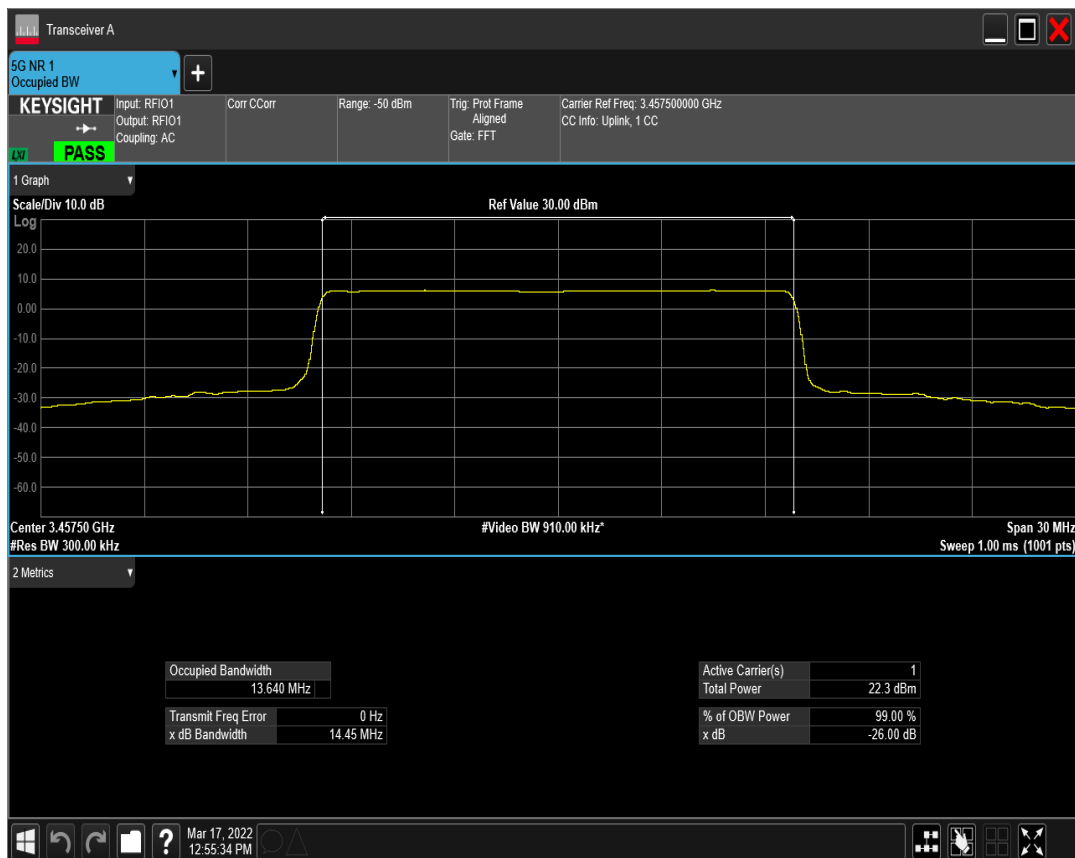
n77(3450-3550) SCS=30kHz DFT_BPSK BW=15MHz Channel=633334 RB=36@0
