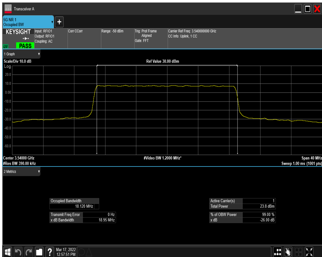
n77(3450-3550) SCS=30kHz DFT_QAM16 BW=20MHz Channel=636000 RB=50@0
