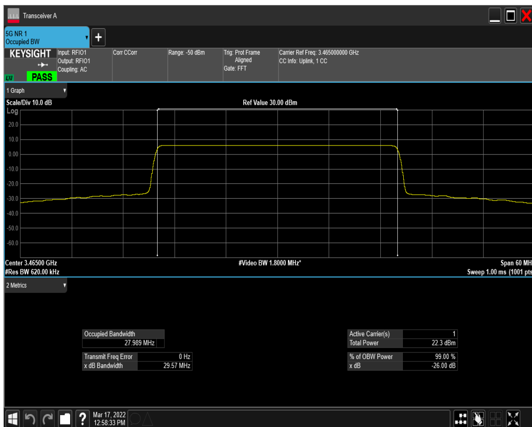
n77(3450-3550) SCS=30kHz DFT_BPSK BW=30MHz Channel=633334 RB=75@0
