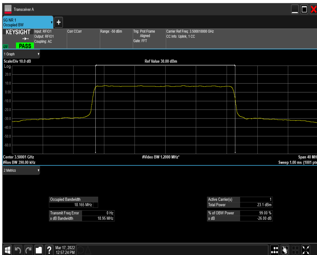
n77(3450-3550) SCS=30kHz DFT_QAM64 BW=20MHz Channel=633334 RB=50@0
