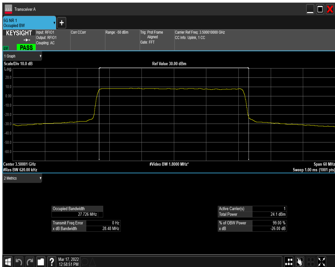
n77(3450-3550) SCS=30kHz DFT_QAM16 BW=30MHz Channel=633334 RB=75@0
