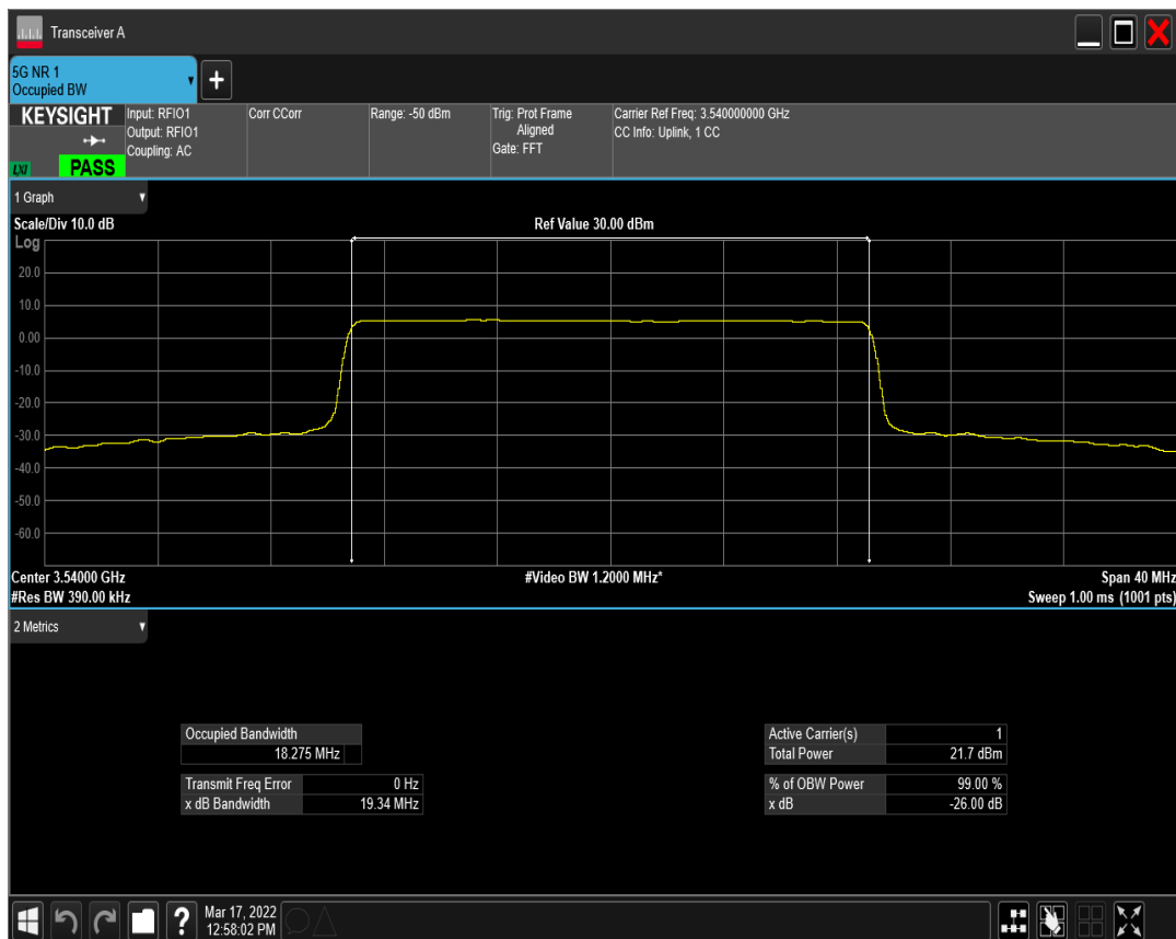
n77(3450-3550) SCS=30kHz DFT_BPSK BW=30MHz Channel=631000 RB=75@0
