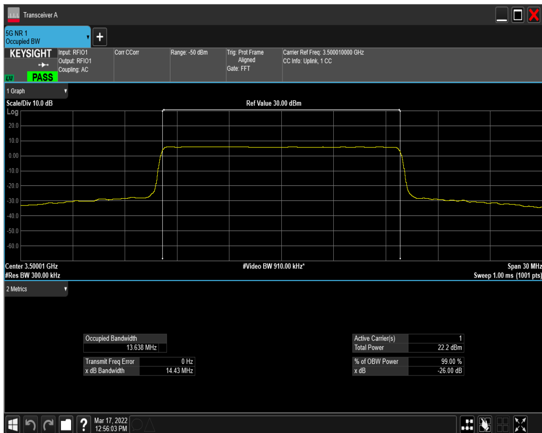
n77(3450-3550) SCS=30kHz DFT_BPSK BW=15MHz Channel=636166 RB=36@0
