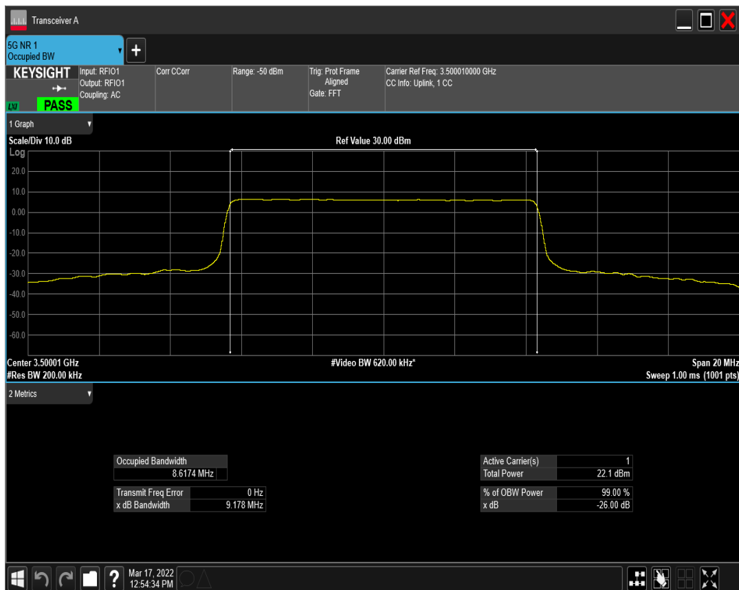
n77(3450-3550) SCS=30kHz DFT_BPSK BW=10MHz Channel=636332 RB=24@0
