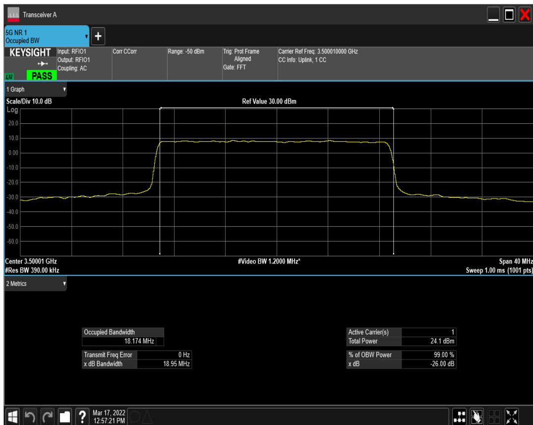
n77(3450-3550) SCS=30kHz DFT_QAM16 BW=20MHz Channel=633334 RB=50@0
