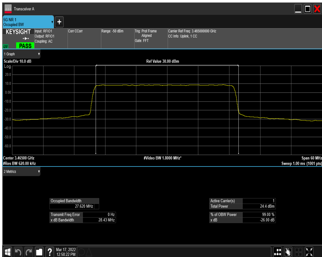
n77(3450-3550) SCS=30kHz DFT_QAM16 BW=30MHz Channel=631000 RB=75@0
