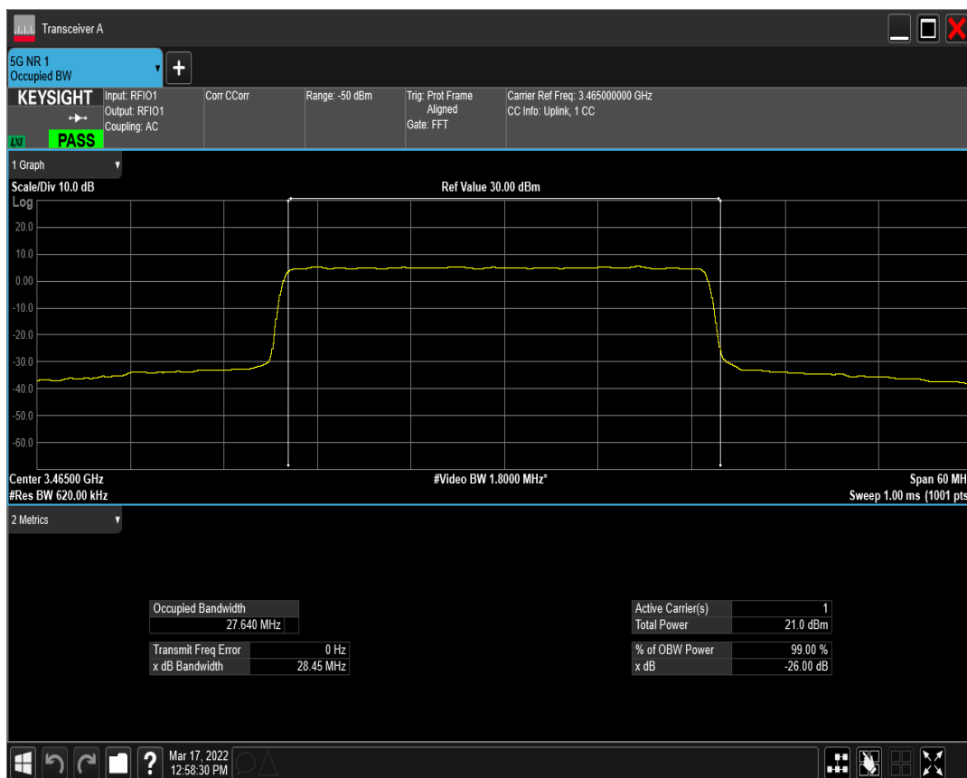
n77(3450-3550) SCS=30kHz CP_QPSK BW=30MHz Channel=631000 RB=78@0
