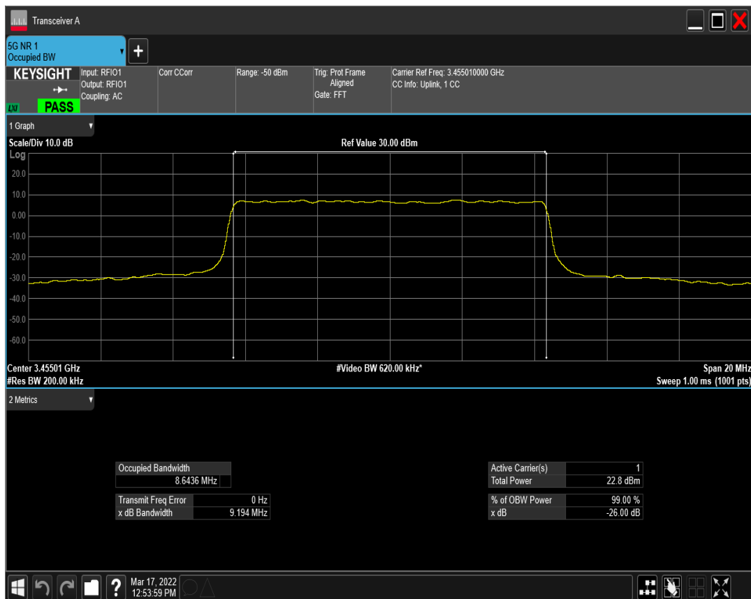
n77(3450-3550) SCS=30kHz DFT_QAM256 BW=10MHz Channel=630334 RB=24@0
