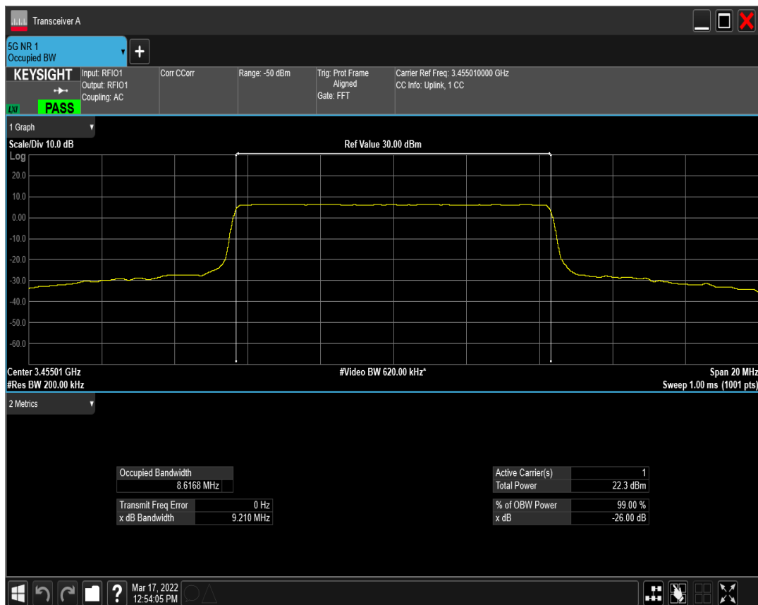
n77(3450-3550) SCS=30kHz DFT_BPSK BW=10MHz Channel=633334 RB=24@0
