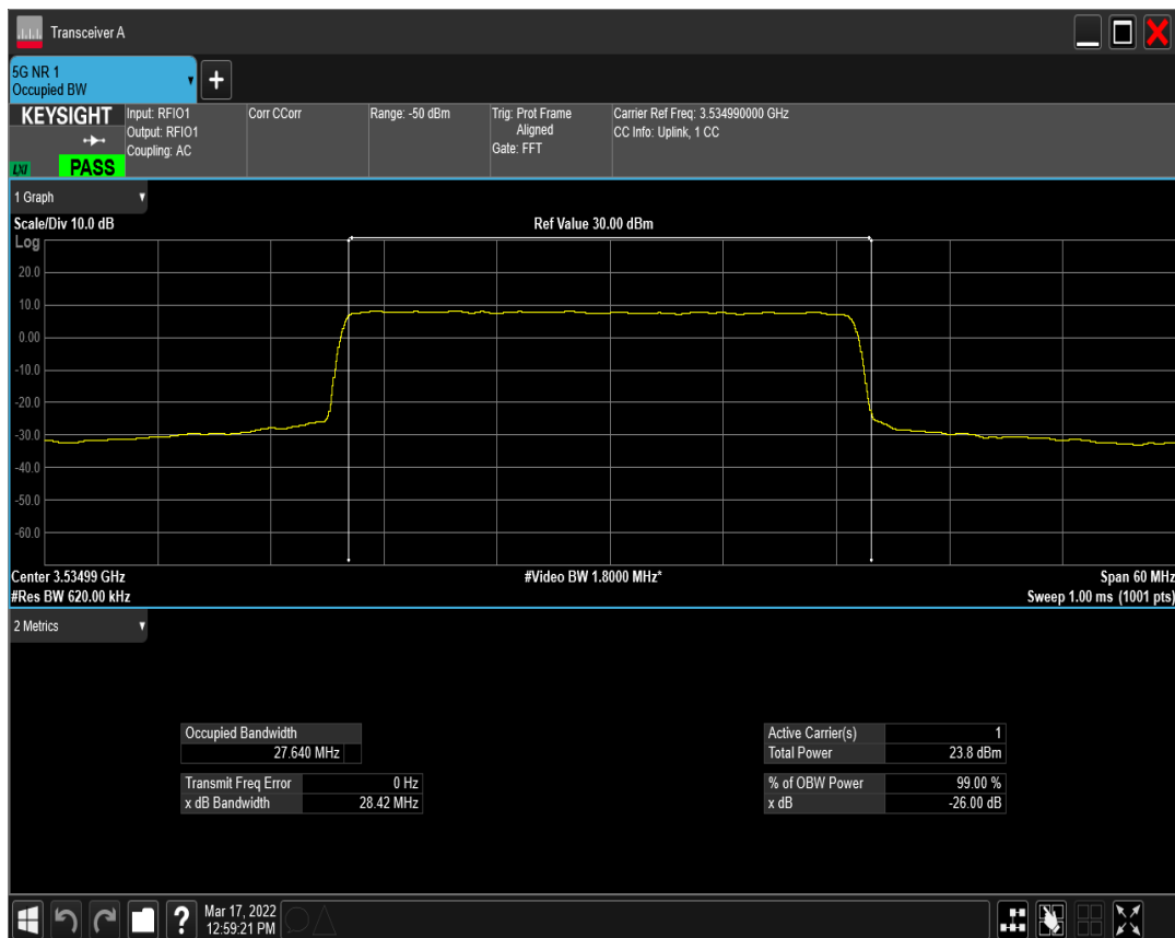
n77(3450-3550) SCS=30kHz DFT_QAM16 BW=30MHz Channel=635666 RB=75@0
