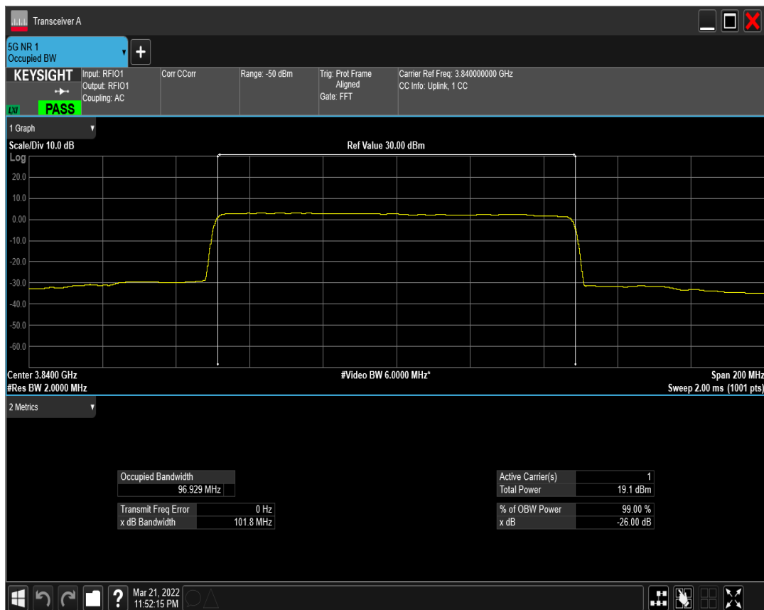
n77(3700-3980) SCS=30kHz CP_QPSK BW=100MHz Channel=656000 RB=273@0
