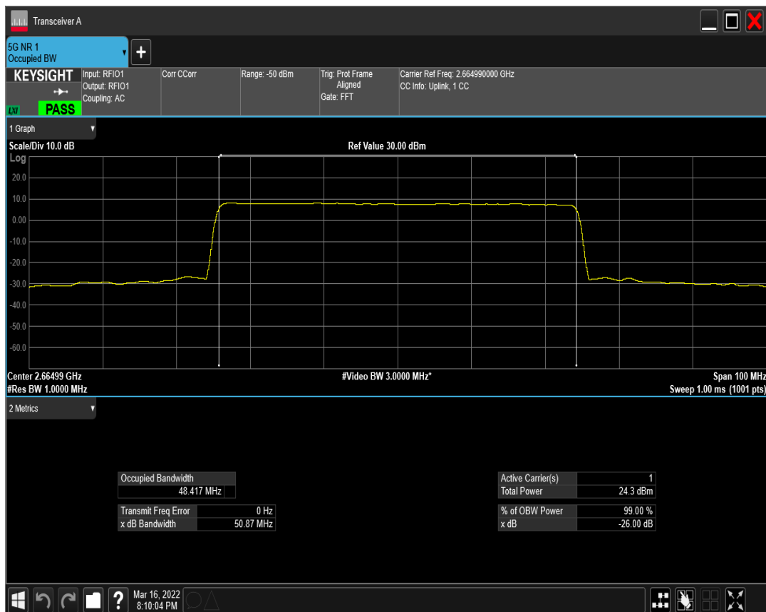
n41 SCS=15kHz DFT_QAM16 BW=50MHz Channel=532998 RB=270@0
