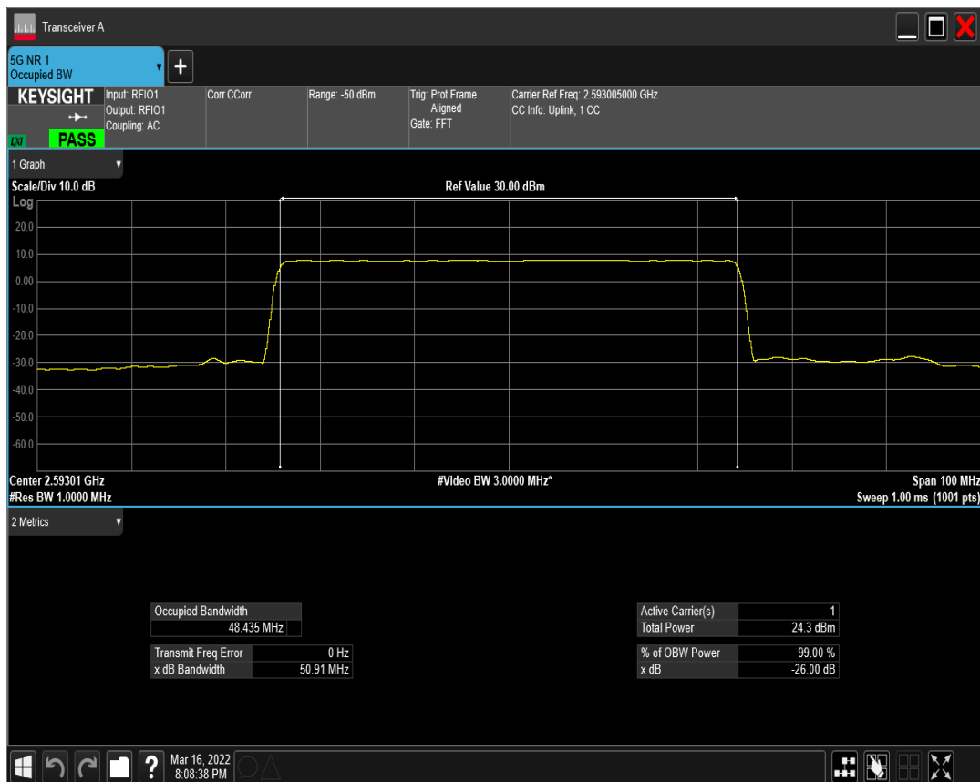
n41 SCS=15kHz DFT_QAM16 BW=50MHz Channel=518601 RB=270@0
