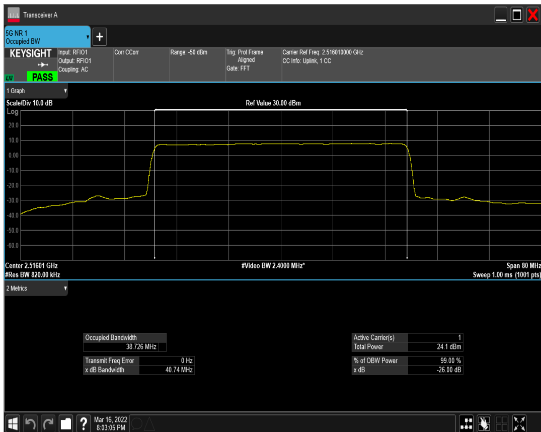
n41 SCS=15kHz DFT_QAM16 BW=40MHz Channel=503202 RB=216@0
