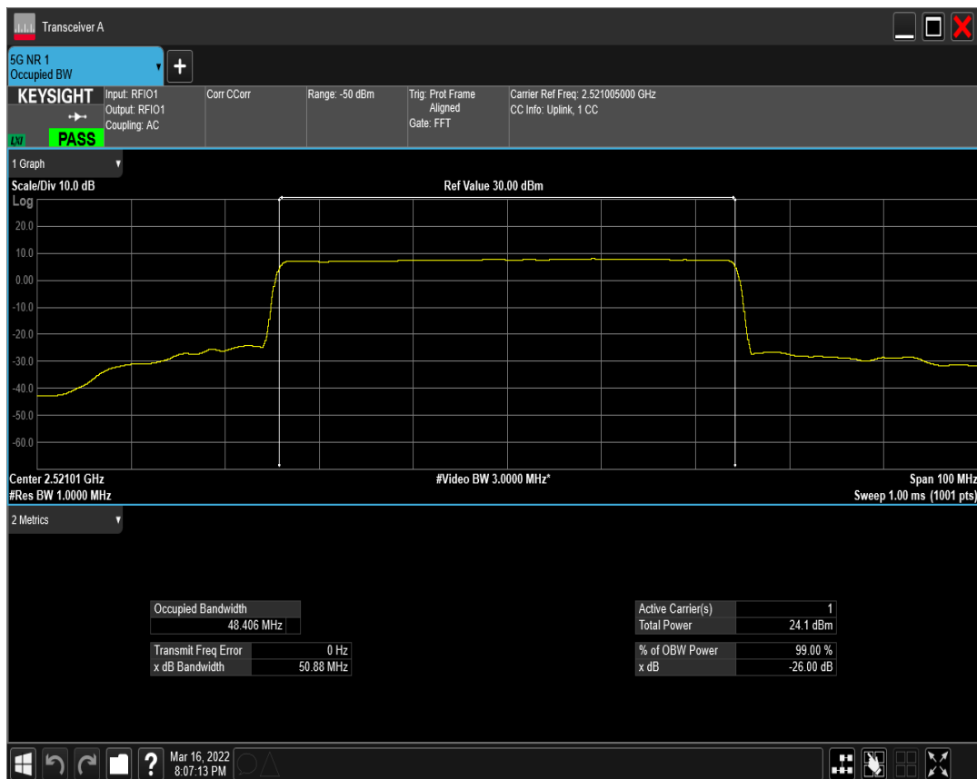
n41 SCS=15kHz DFT_QAM16 BW=50MHz Channel=504201 RB=270@0
