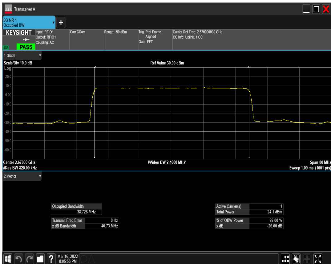
n41 SCS=15kHz DFT_QAM16 BW=40MHz Channel=534000 RB=216@0
