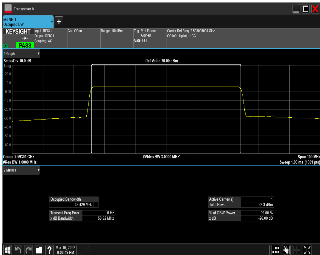
n41 SCS=15kHz DFT_BPSK BW=50MHz Channel=532998 RB=270@0
