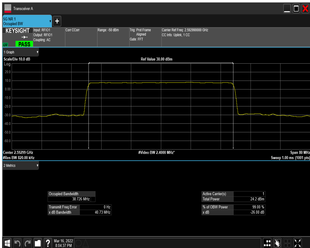
n41 SCS=15kHz DFT_QAM16 BW=40MHz Channel=518598 RB=216@0
