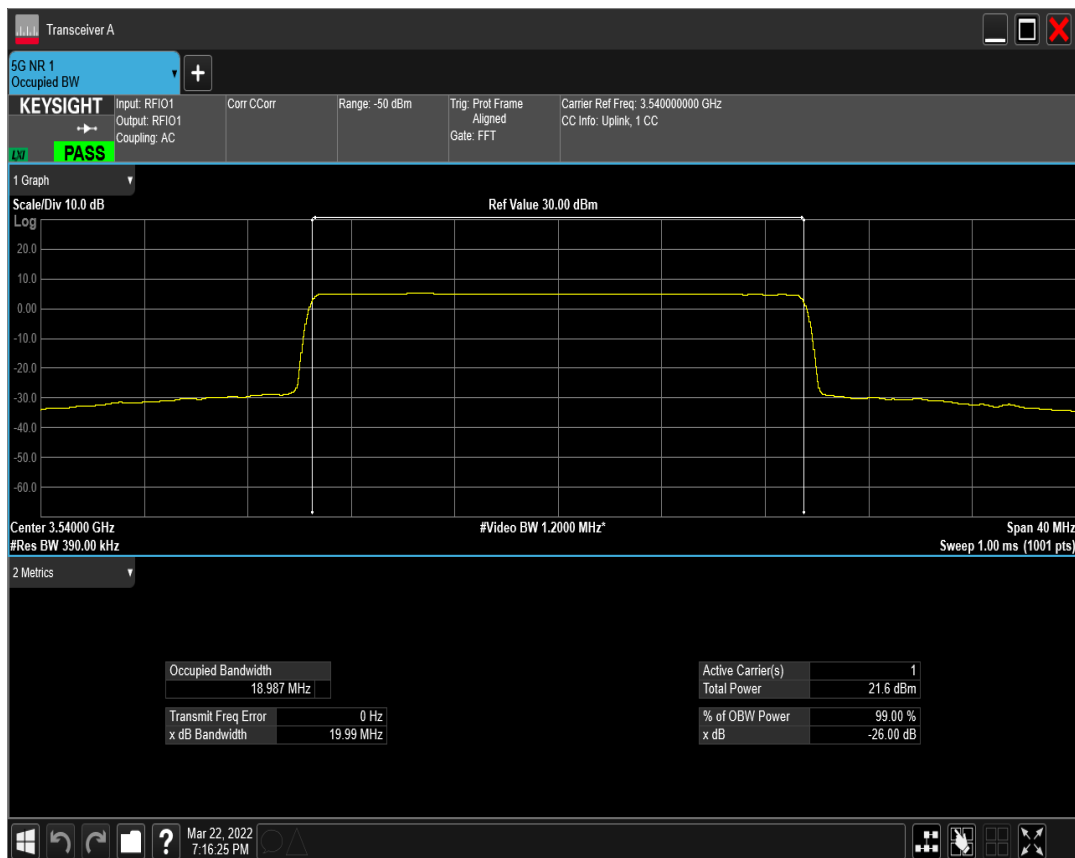
n77(3450-3550) SCS=15kHz DFT_BPSK BW=30MHz Channel=631000 RB=160@0
