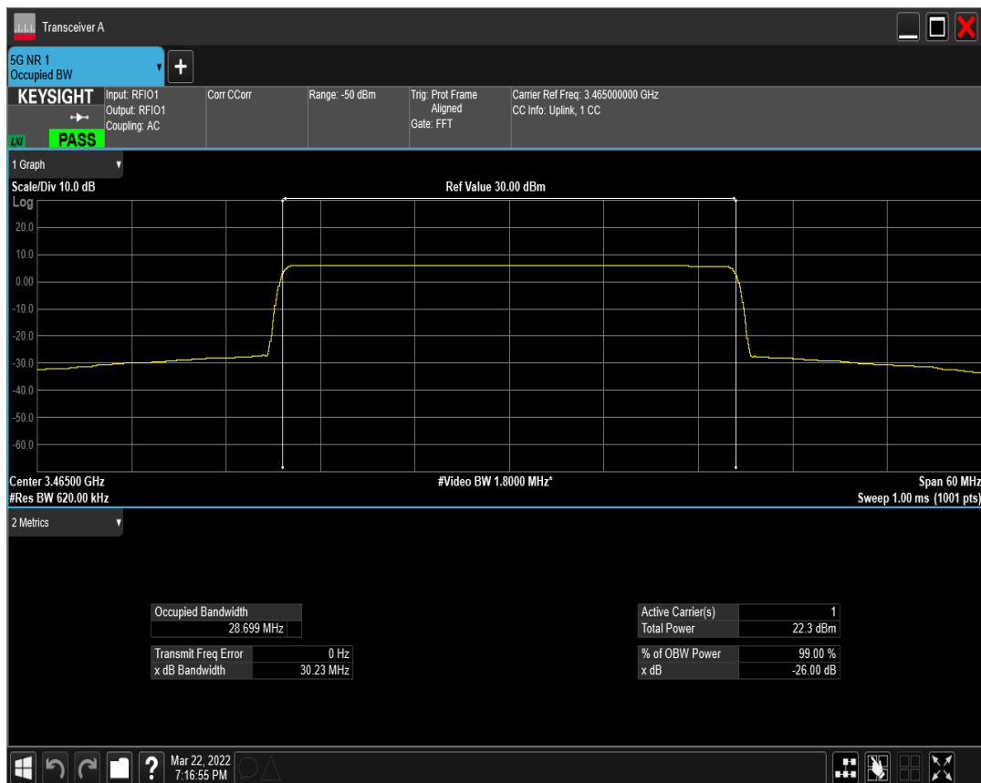
n77(3450-3550) SCS=15kHz DFT_BPSK BW=30MHz Channel=633334 RB=160@0
