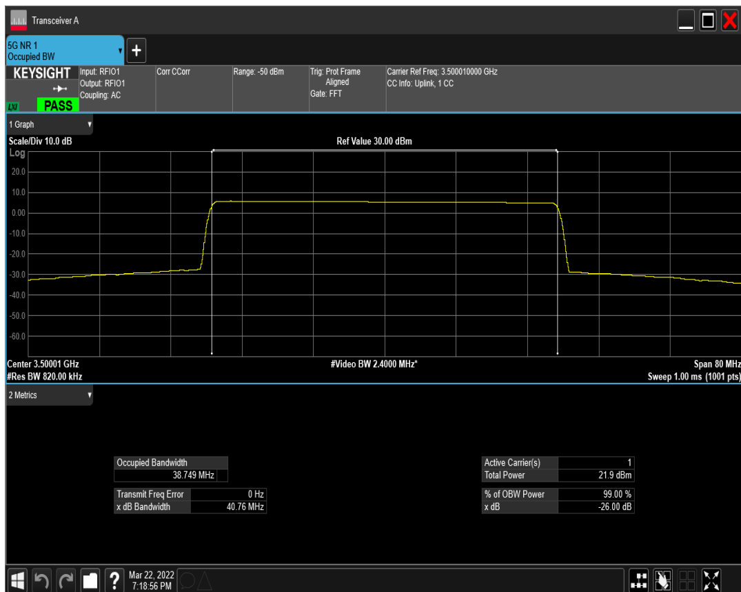
n77(3450-3550) SCS=15kHz DFT_BPSK BW=40MHz Channel=635332 RB=216@0
