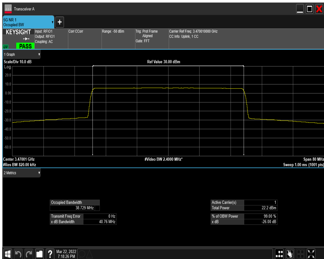
n77(3450-3550) SCS=15kHz DFT_BPSK BW=40MHz Channel=633334 RB=216@0
