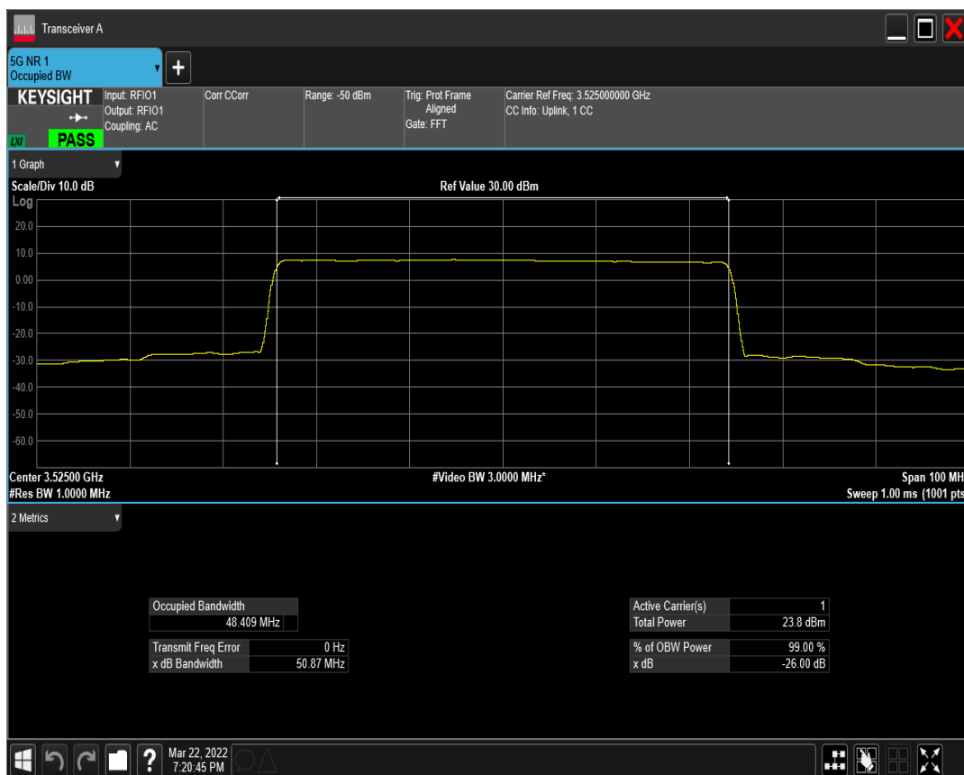
n77(3450-3550) SCS=15kHz DFT_QAM16 BW=50MHz Channel=635000 RB=270@0
