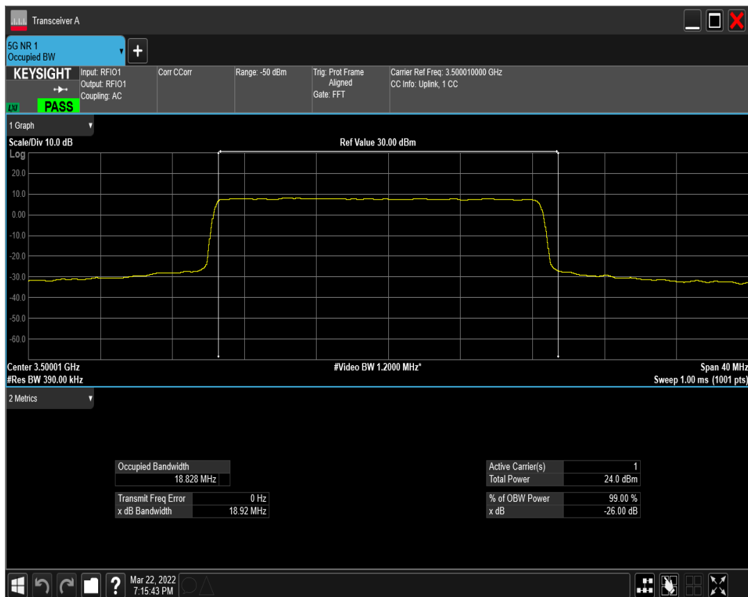
n77(3450-3550) SCS=15kHz DFT_QAM16 BW=20MHz Channel=633334 RB=100@0
