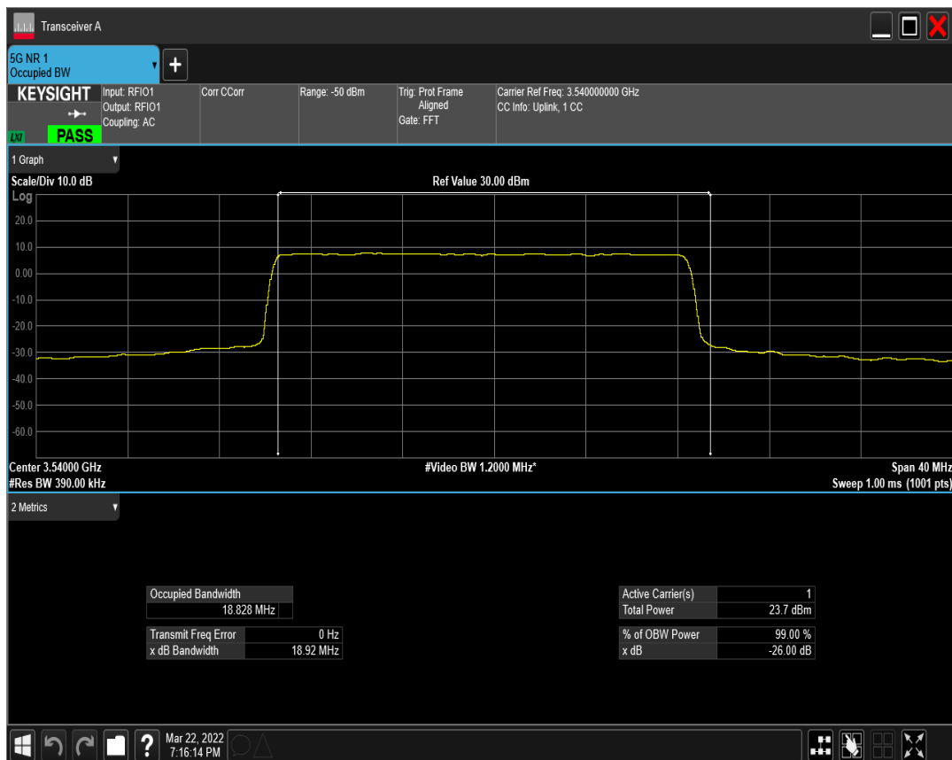
n77(3450-3550) SCS=15kHz DFT_QAM16 BW=20MHz Channel=636000 RB=100@0
