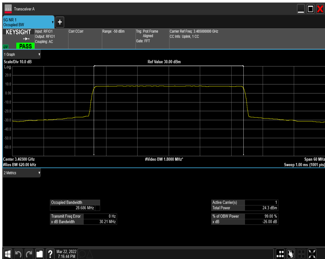
n77(3450-3550) SCS=15kHz DFT_QAM16 BW=30MHz Channel=631000 RB=160@0
