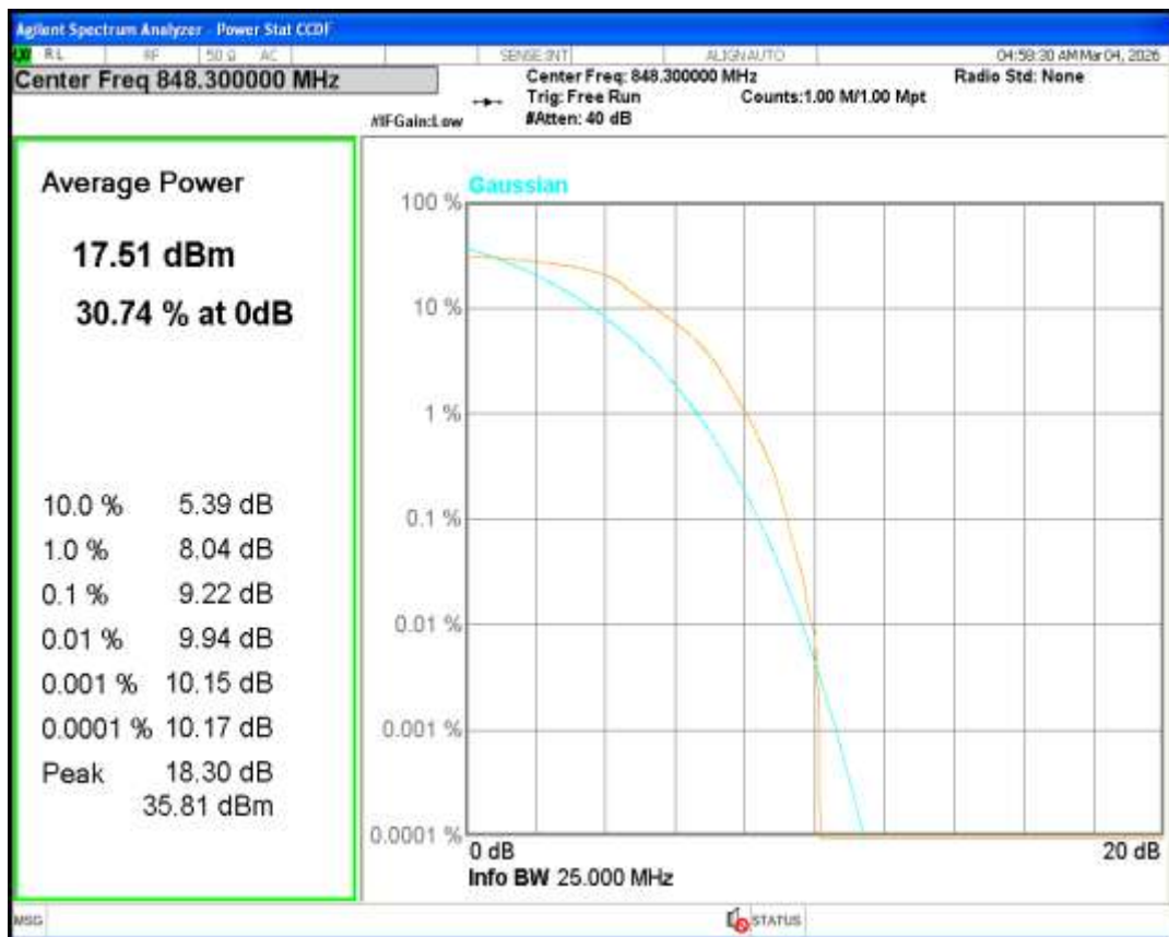
Band26(824-849) QPSK BW=10MHz Channel=26840 RB Size=6 Position=#0 NB Index=0
