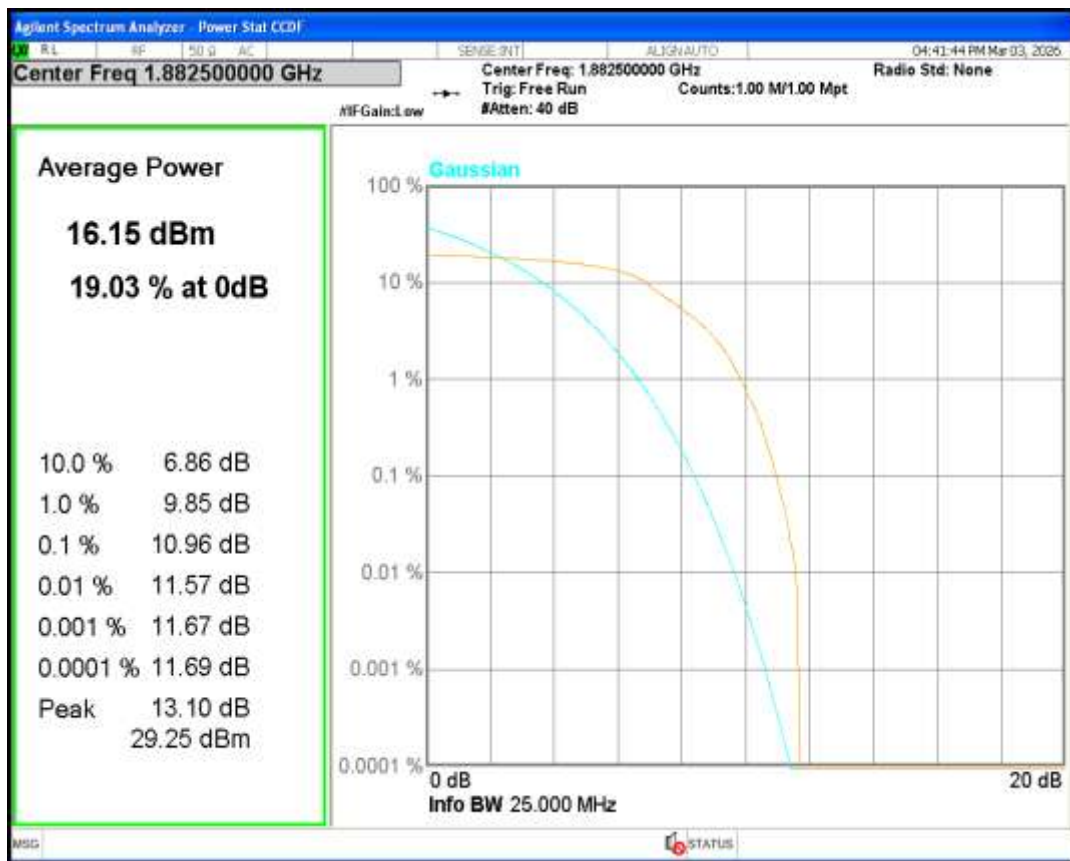
Band25 QPSK BW=5MHz Channel=26665 RB Size=6 Position=#0 NB Index=0
