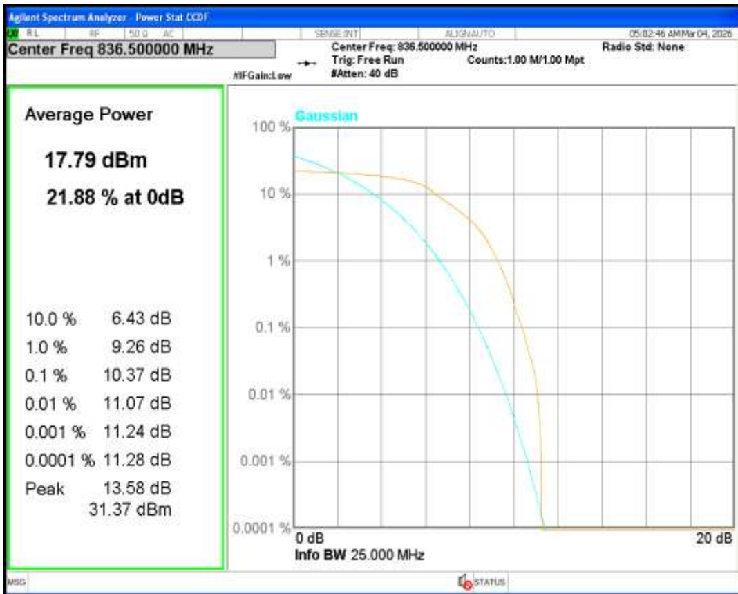
Band26(824-849) QPSK BW=15MHz Channel=26965 RB Size=6 Position=#0 NB Index=0
