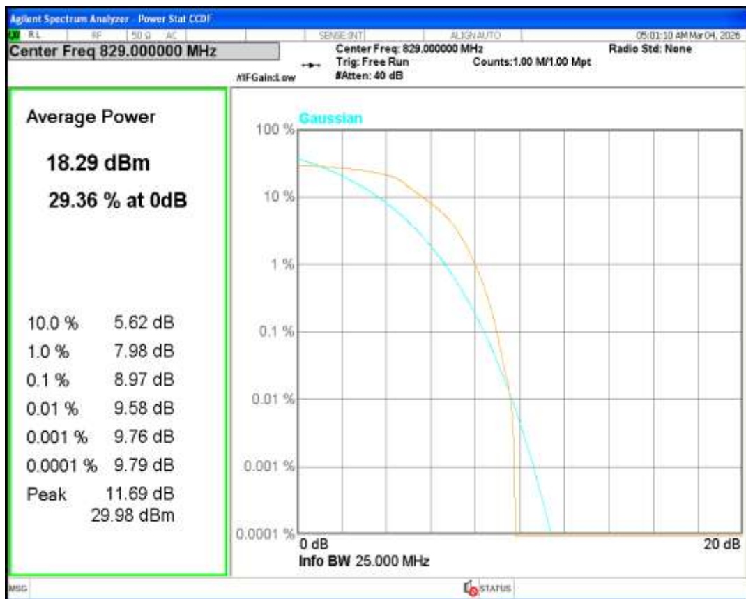
Band26(824-849) QPSK BW=10MHz Channel=26915 RB Size=6 Position=#0 NB Index=0
