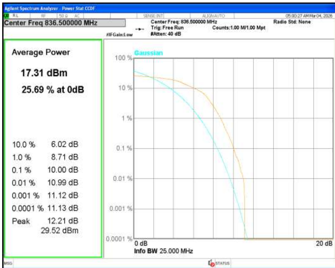
Band26(824-849) QPSK BW=1.4MHz Channel=26797 RB Size=6 Position=#0 NB Index=0
