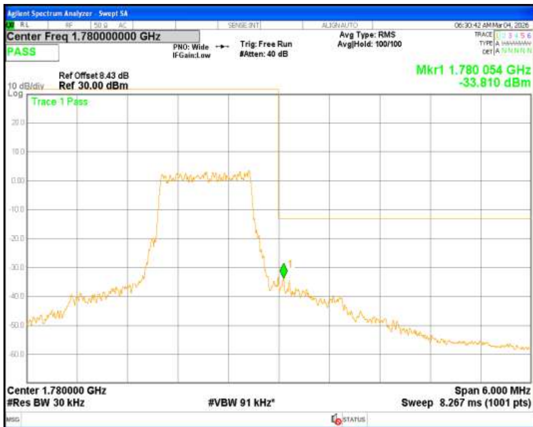
Band66 QPSK BW=5MHz Channel=131997 RB Size=1 Position=#0 NB Index=0
