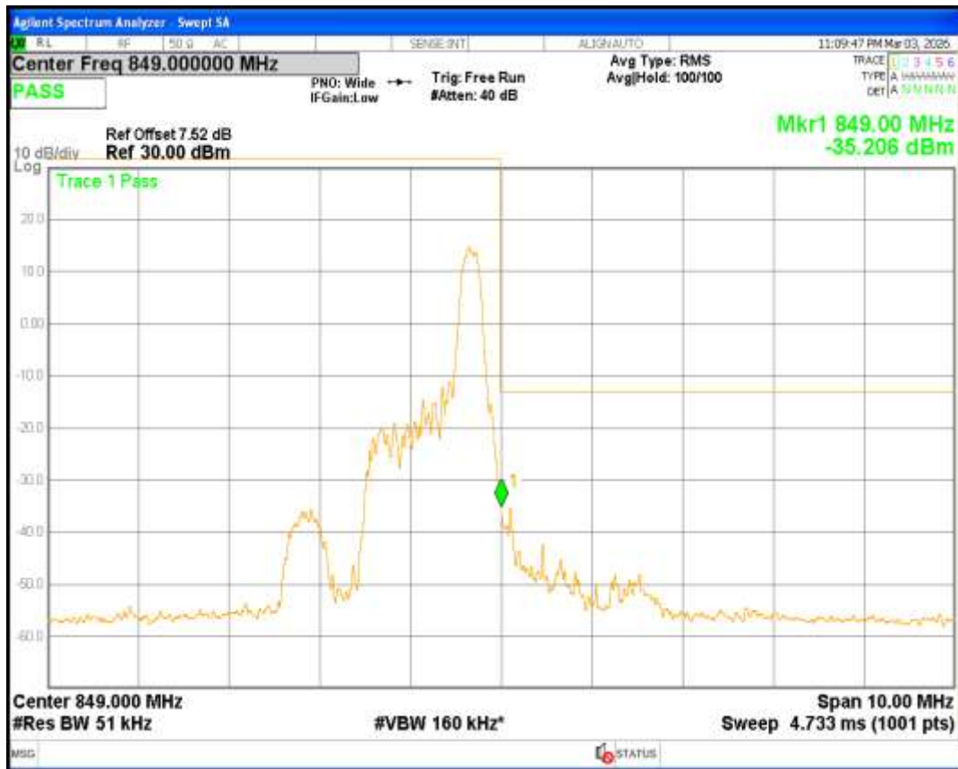
Band5 QPSK BW=5MHz Channel=20625 RB Size=6 Position=#Max NB Index=3
