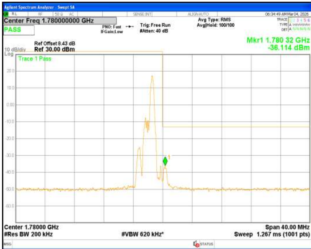
Band66 16QAM BW=20MHz Channel=132572 RB Size=5 Position=#Max NB Index=15
