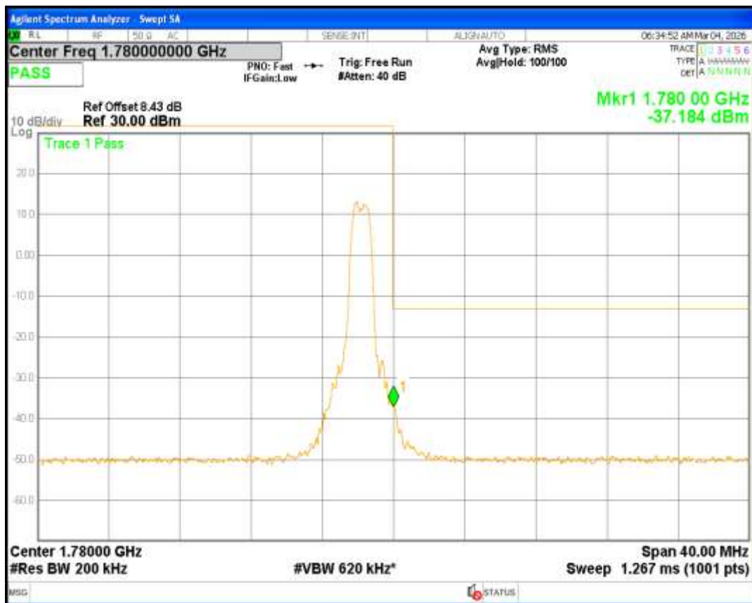
Band66 16QAM BW=3MHz Channel=131987 RB Size=1 Position=#0 NB Index=0
