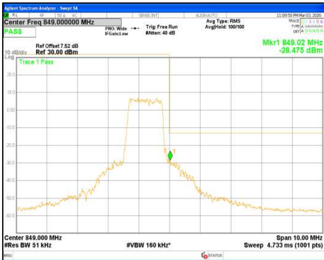
Band66 16QAM BW=1.4MHz Channel=131979 RB Size=1 Position=#0 NB Index=0
