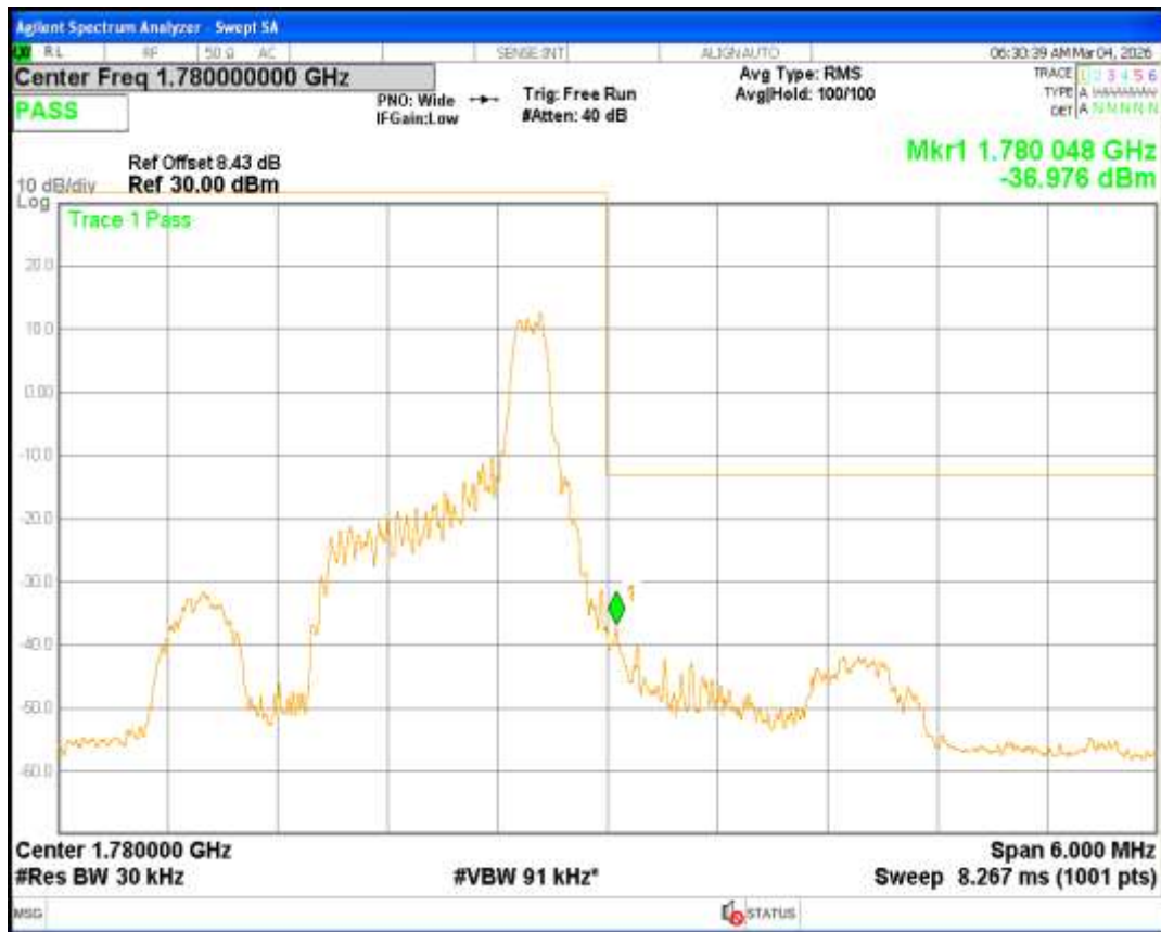
Band66 QPSK BW=3MHz Channel=132657 RB Size=6 Position=#Max NB Index=1
