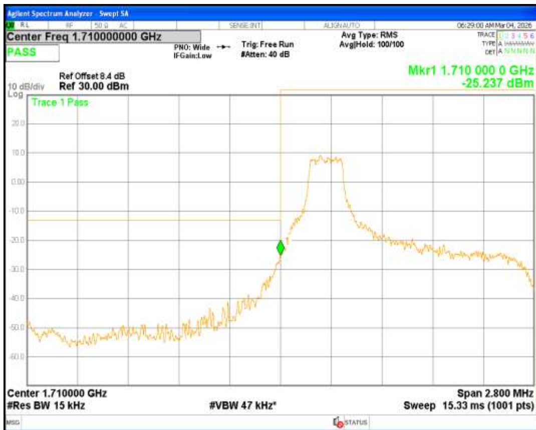
Band66 16QAM BW=5MHz Channel=132647 RB Size=5 Position=#Max NB Index=3
