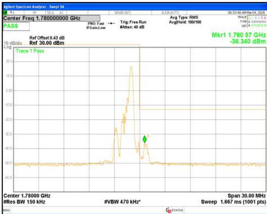
Band66 16QAM BW=15MHz Channel=132597 RB Size=5 Position=#Max NB Index=1
