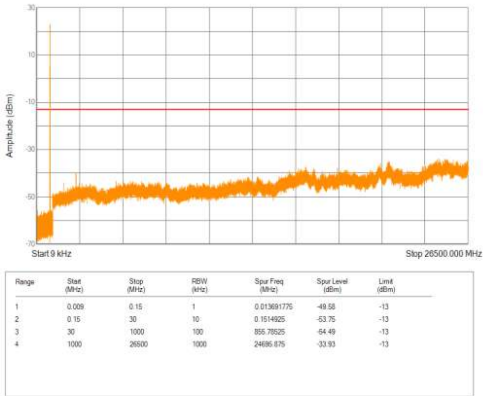
Band5 16QAM BW=10MHz Channel=20450 RB Size=1 Position=#0 NB Index=0
