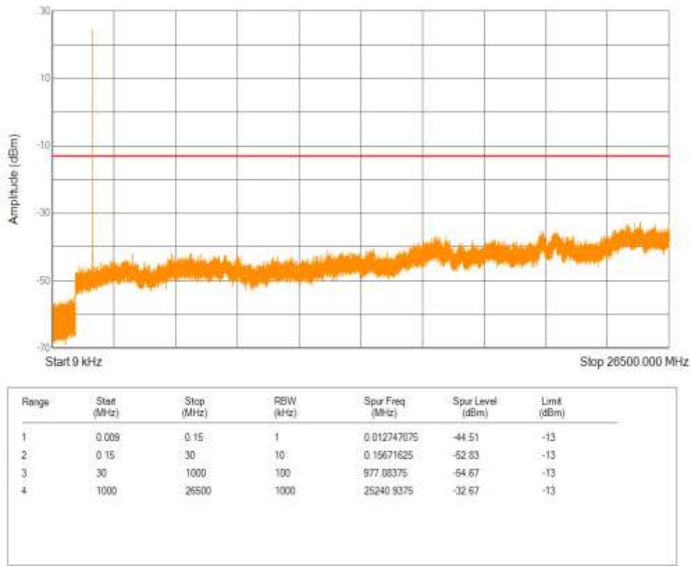
Band4 QPSK BW=5MHz Channel=20175 RB Size=6 Position=#0 NB Index=0
