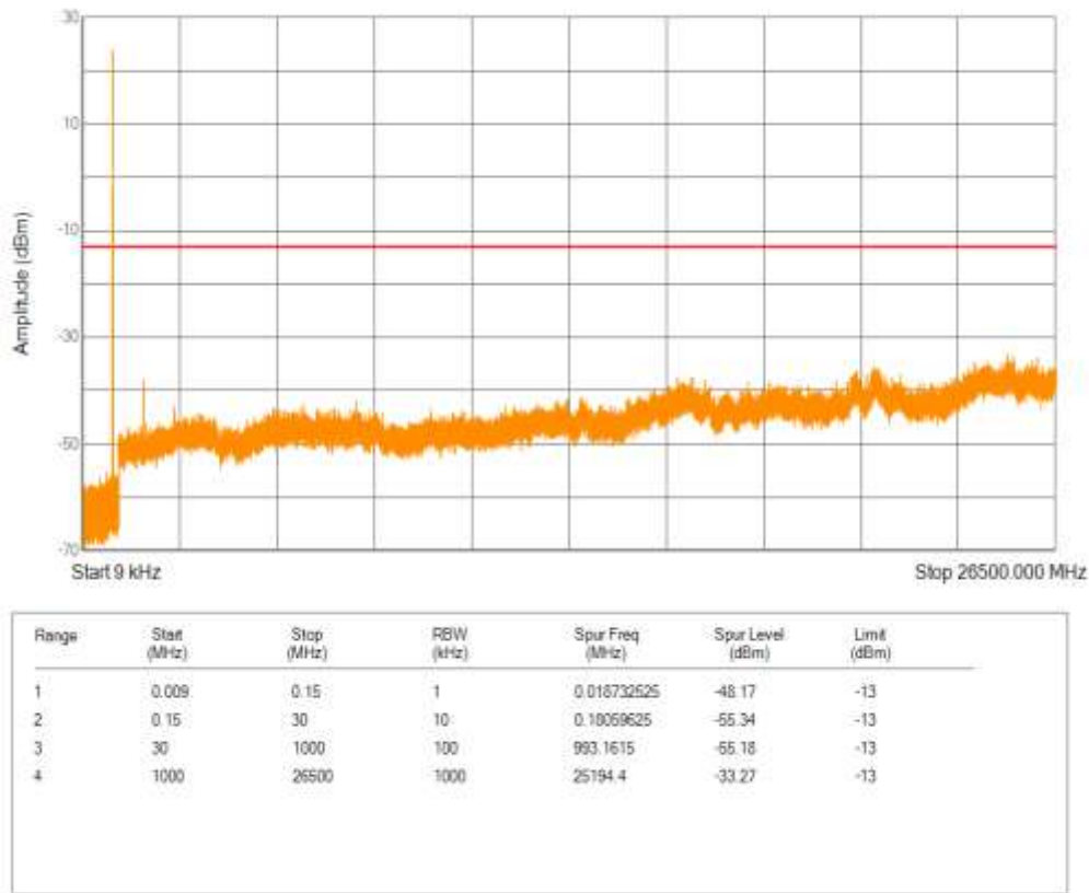
Band5 16QAM BW=10MHz Channel=20525 RB Size=5 Position=#0 NB Index=0
