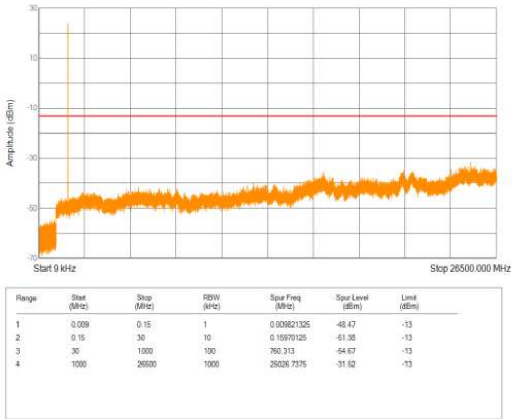
Band66 16QAM BW=15MHz Channel=132322 RB Size=1 Position=#0 NB Index=0
