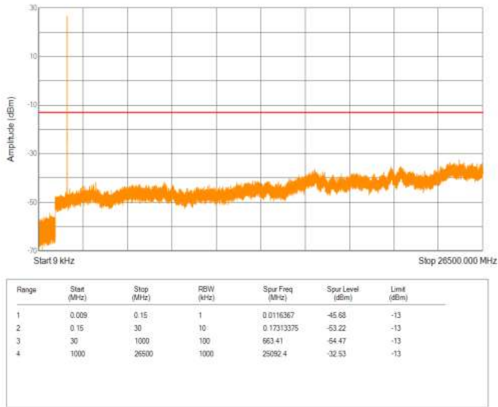
Band66 QPSK BW=20MHz Channel=132322 RB Size=1 Position=#0 NB Index=0
