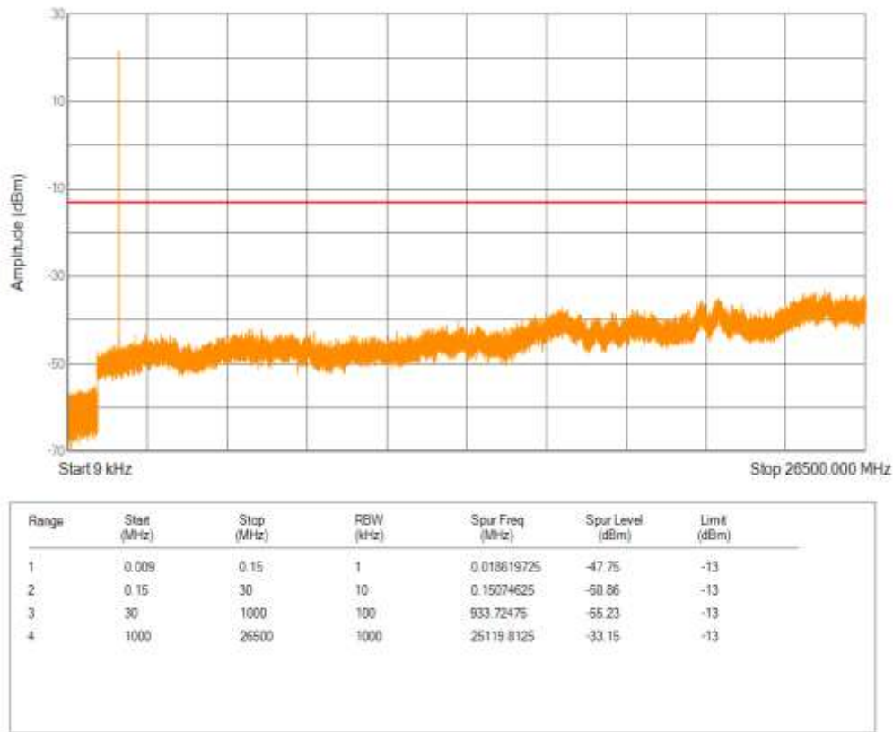
Band4 QPSK BW=3MHz Channel=20175 RB Size=1 Position=#0 NB Index=0
