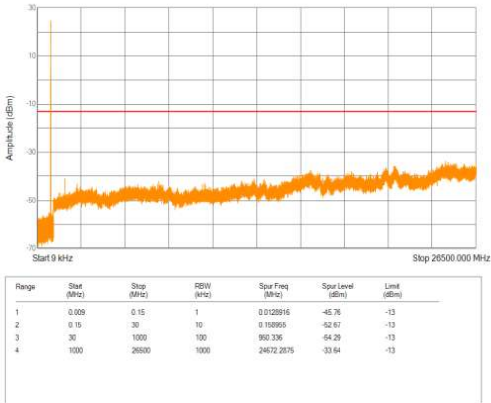
Band5 QPSK BW=5MHz Channel=20525 RB Size=1 Position=#0 NB Index=0
