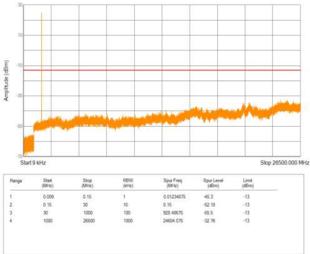
Band66 QPSK BW=10MHz Channel=132622 RB Size=1 Position=#0 NB Index=0
