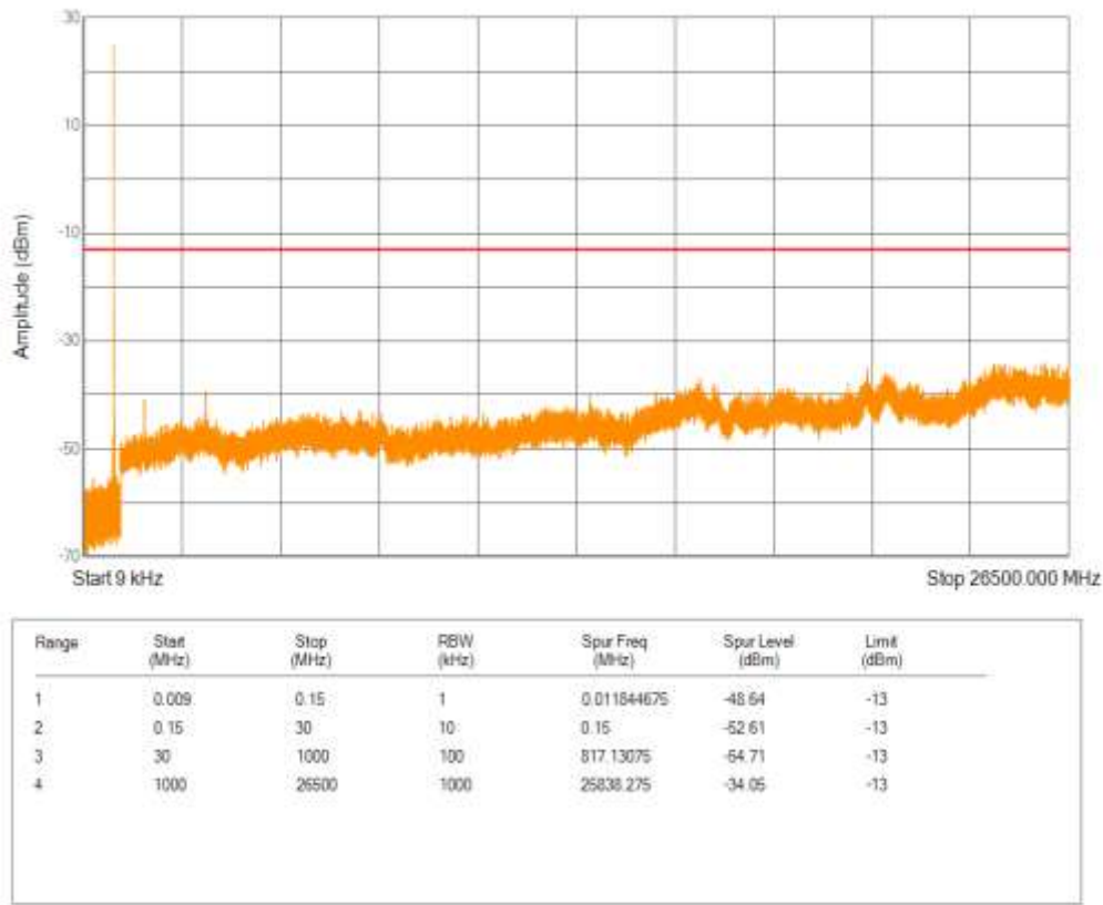
Band5 16QAM BW=1.4MHz Channel=20407 RB Size=5 Position=#0 NB Index=0
