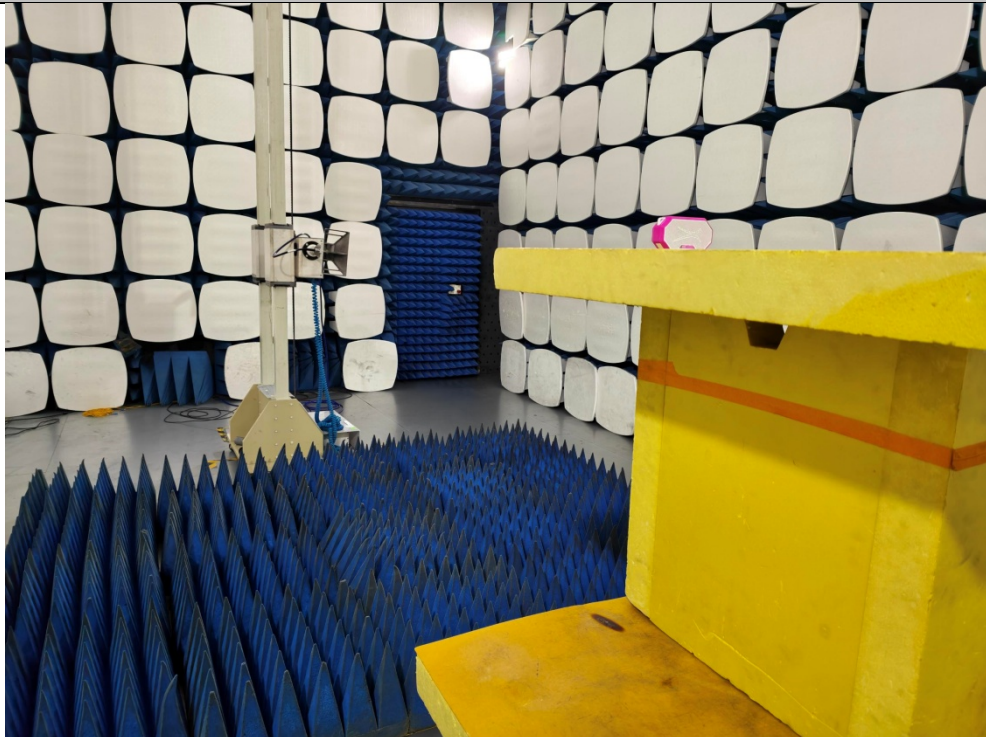
Radiated Spurious Emission, Above 1GHz
