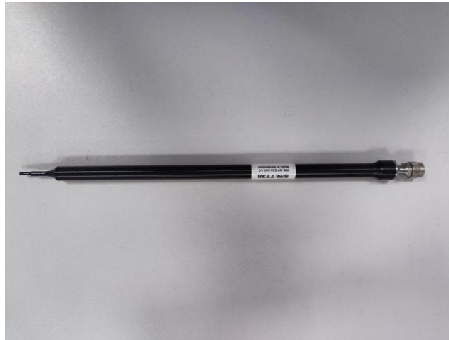
Figure 1-Speag COMOSAR Dosimetric E field Dipole
