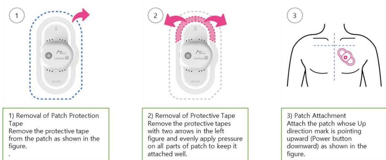
Figure 11.2. How to attach ATP-C130
