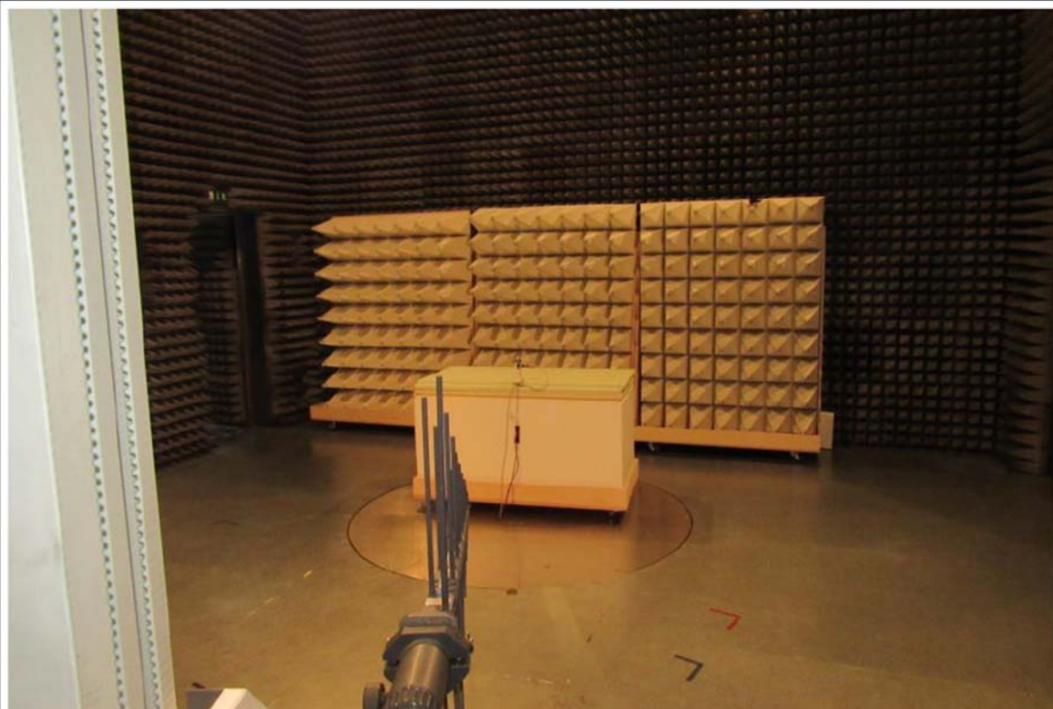
Test setup radiated between 200MHz and 1GHz
