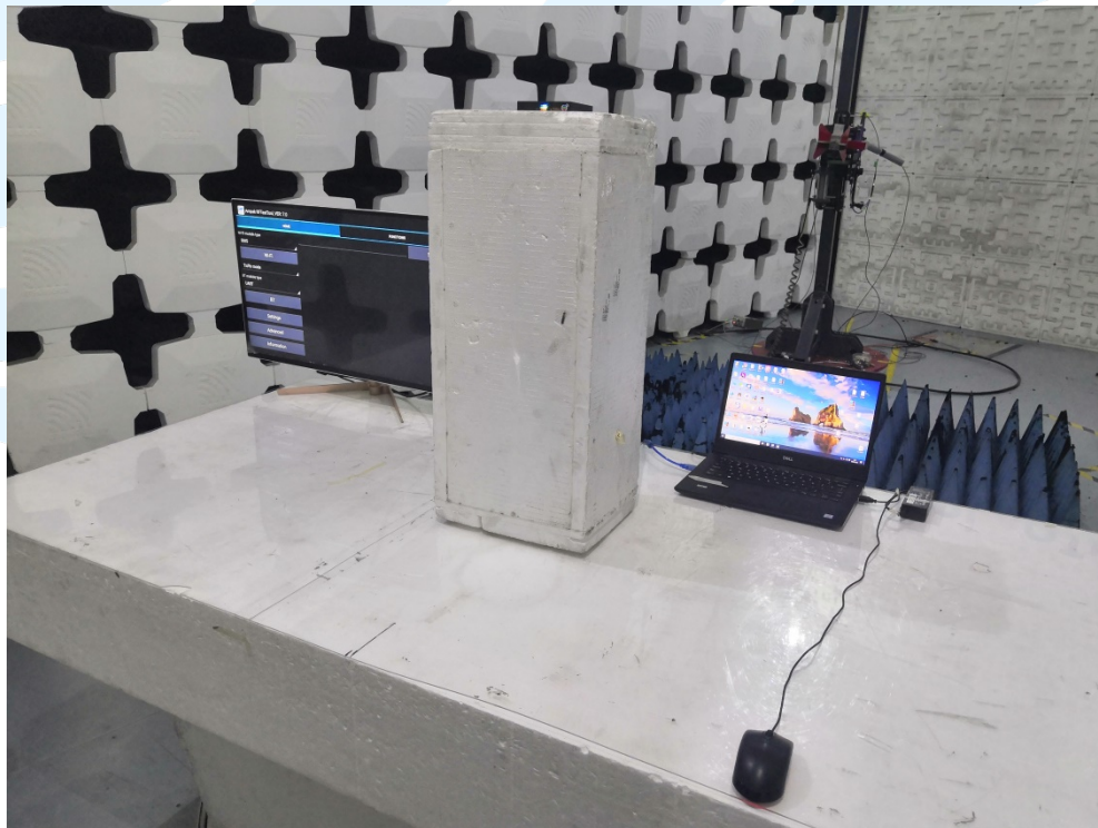
Radiated emission Test Setup (Above 1 GHz)
