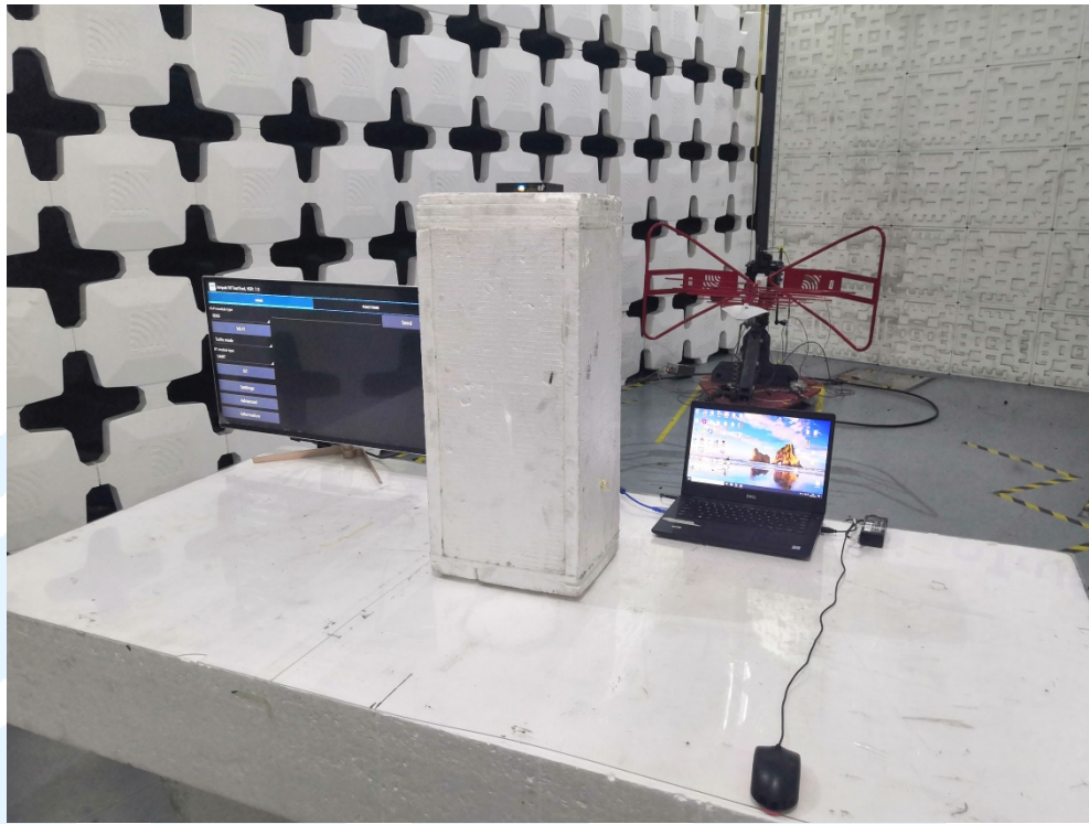
Radiated emission Test Setup (30 MHz~1 GHz)
