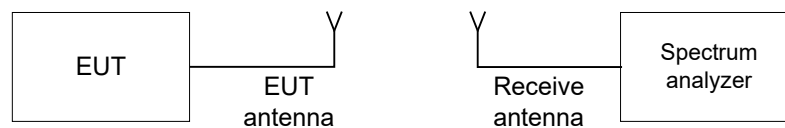
Figure 7.4.1 Band edge emission test setup
