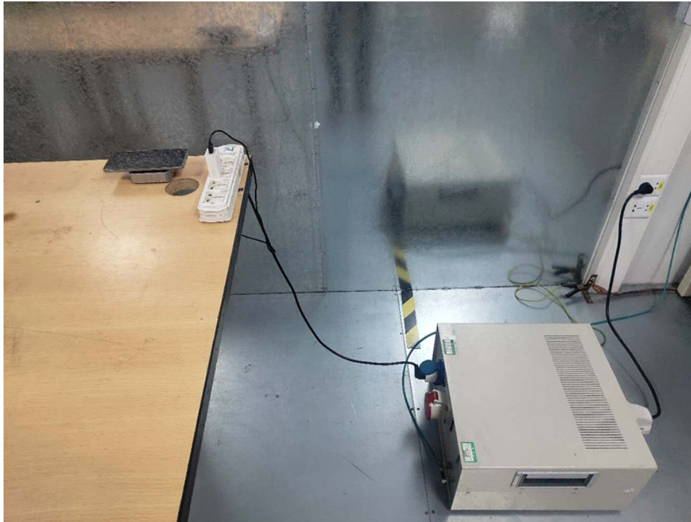
Conducted Emission Test Setup:
