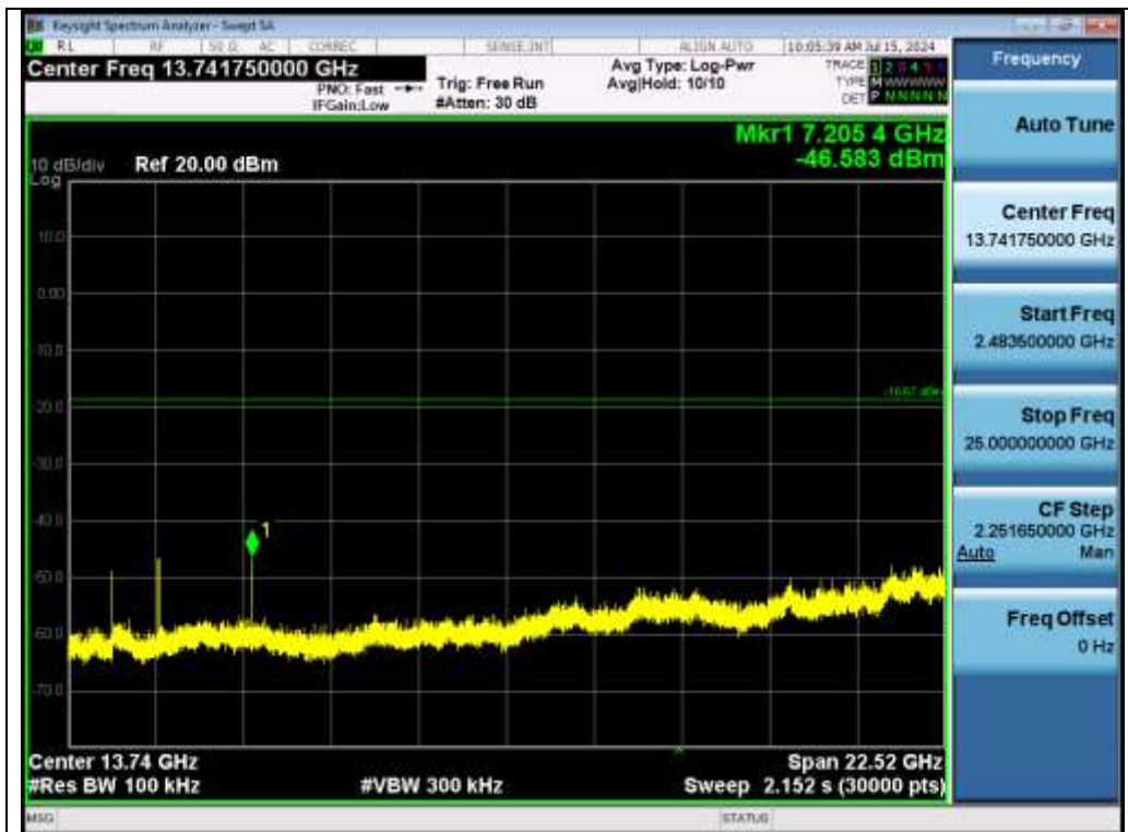
Test_Graph_BR_ANT1_2402_1Mbps_Higher Band Emissions
