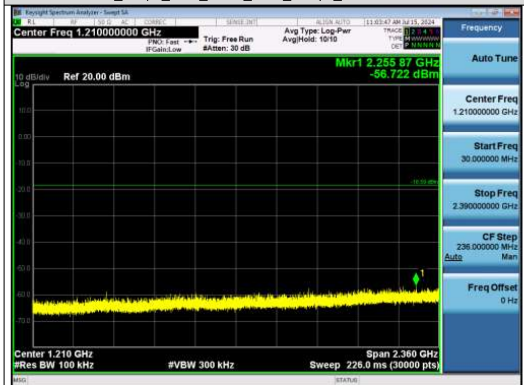
Test Graph EDR ANT1 2402 3Mbps Lower Band Emissions
