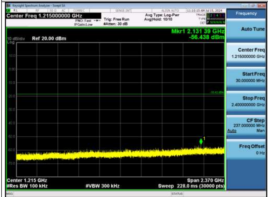
Test_Graph_EDR_ANT1_2480_3Mbps_Lower Band Emissions
