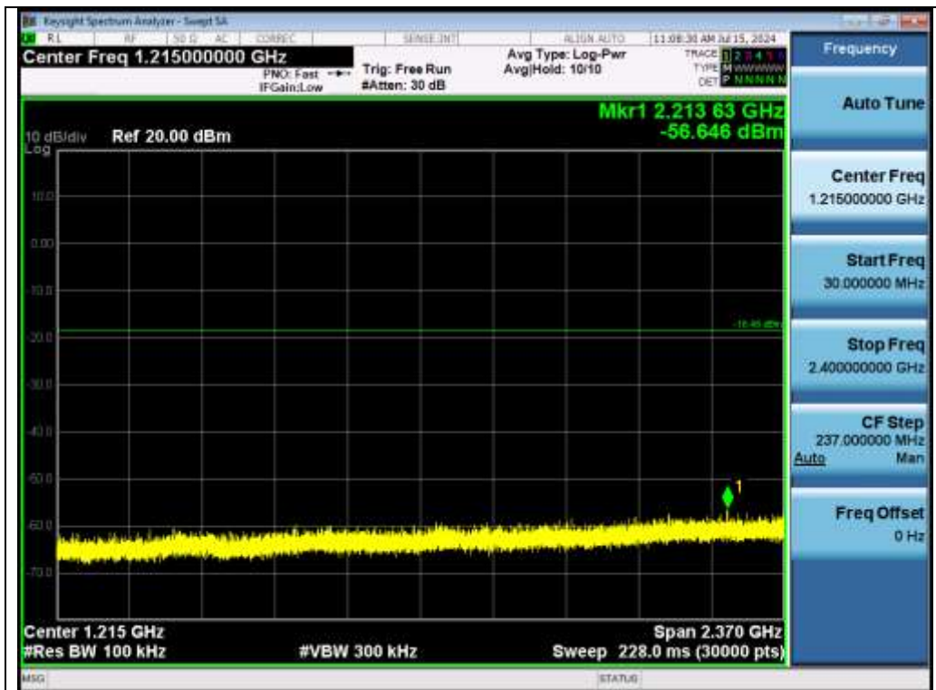
Test_Graph_EDR_ANT1_2441_3Mbps_Lower Band Emissions
