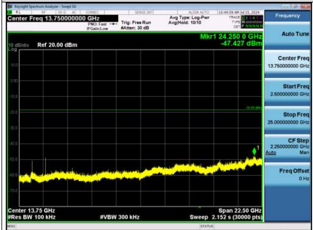
Test_Graph_EDR_ANT1_2480_2Mbps_Higher Band Emissions
