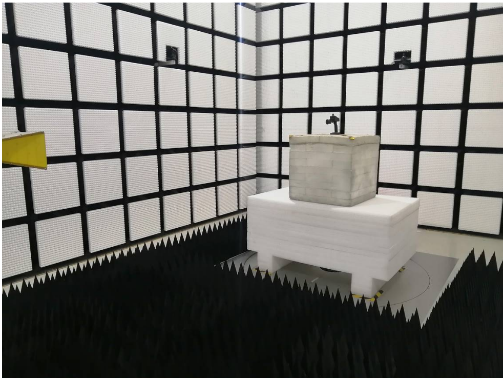
Radiated Emission Above 1GHz View
