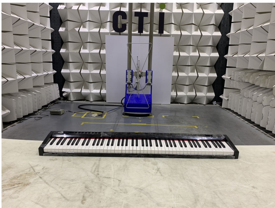
Radiated spurious emission Test Setup-1(Below 1GHz)
