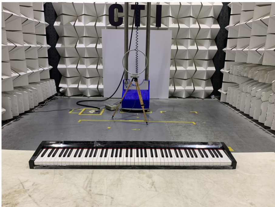
Radiated spurious emission Test Setup-1(Below 30MHz)
