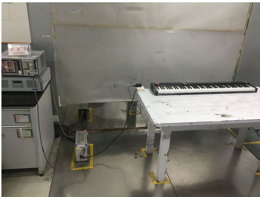
Radiated spurious emission Test Setup-2(CE)
